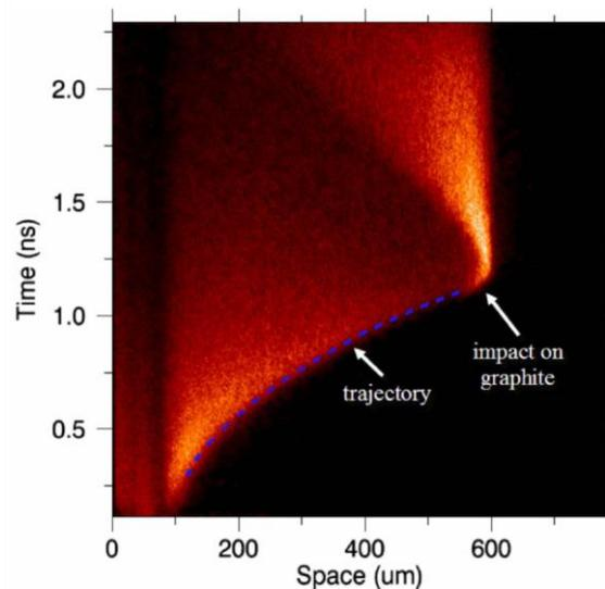
Figure 2: Side-on streaked image of x-ray self-emission from highly accelerated CH foil. Laser from the left side of image drives the foil into a stationary graphite target on right. Velocity before impact is  $1040 \pm 60$  km/s.
