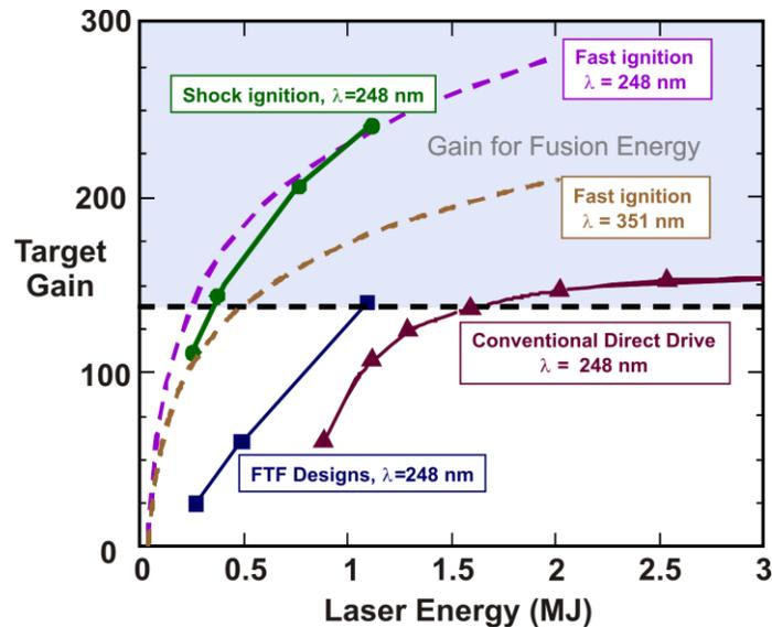
Figure 1: Gain curves from 1D simulations of various high performance direct drive target designs comparing KrF performance to third harmonic Nd:glass systems. Shaded region shows sufficient gain for pure fusion power plant. Dashed lines represent an analytical prediction for fast ignition. ‘FTF’ designs refer to a particular set of conventional direct drive designs that use high implosion velocity without a shock ignition pulse.
