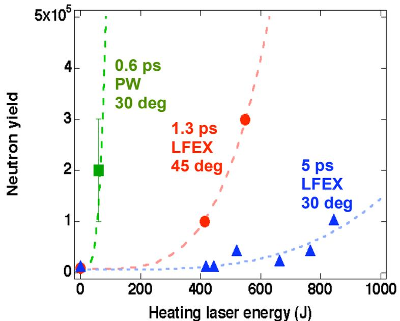
Figure 4. Neutron yield as functions of heating laser energy. Indicated are heating pulse width and opening angle of the used cone.
