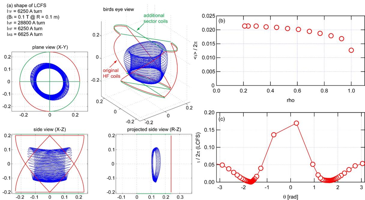
FIG. 10. Flux surface formed using the additional sector coils obtained from the calculation of magnetic field line tracing. (a) Shape of the last closed flux surface (LCFS), (b) radial profile of the averaged rotational transform, and (c) poloidal profile of the rotational transform of LCFS.
