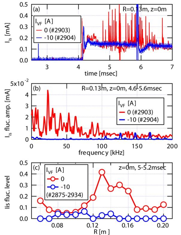
FIG. 9. (a) Temporal evolution and (b) frequency spectrum of the ion saturation current at the location where the fluctuation is largest in the ECH pre-ionized plasma. (c) Radial profile of the fluctuation level evaluated using the standard deviations of the signals divided by the DC values.
