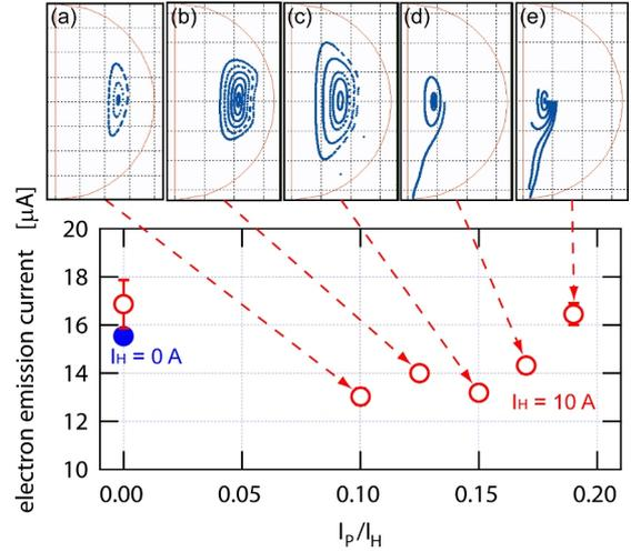
FIG. 4. Dependence of the electron emission current of the electron-emission impedance on magnetic configuration.
