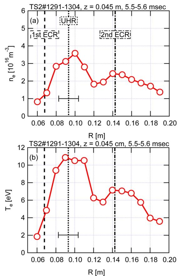
FIG. 7. Radial profiles of (a) electron density and (b) electron temperature of the ECH plasma as the pre-ionized phase of tokamak operation.
