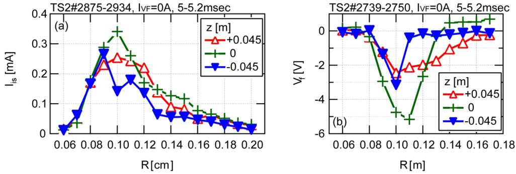
FIG. 8. Radial profiles of (a) ion saturation currents and (b) floating potentials measured using Langmuir probes at  $z = +0.045, 0, -0.045$  m. The midplane corresponds to  $z = 0$  m.
