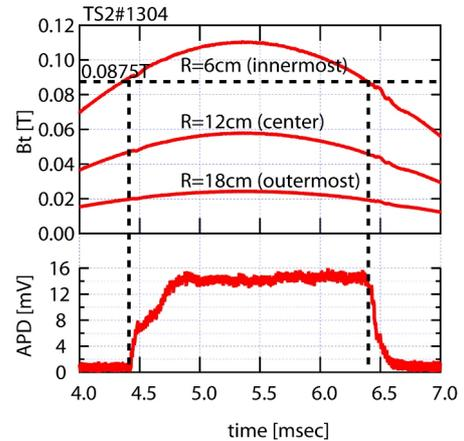
FIG. 6. Temporal evolutions of the toroidal field strength at three locations calculated using the TF coil current (upper) and the intensity of visible emission measured using the avalanche photodiode detector (lower).
