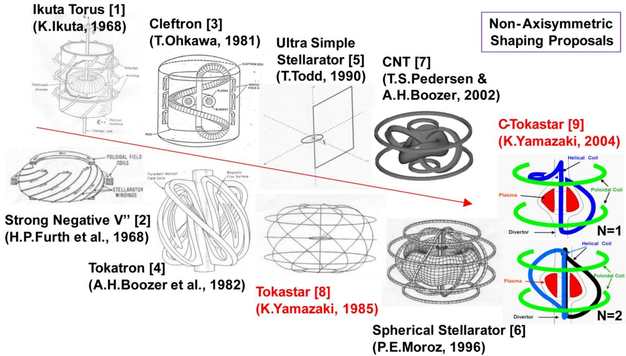
FIG. 1. Proposal of TOKASTAR comparing with other compact helical configurations.
