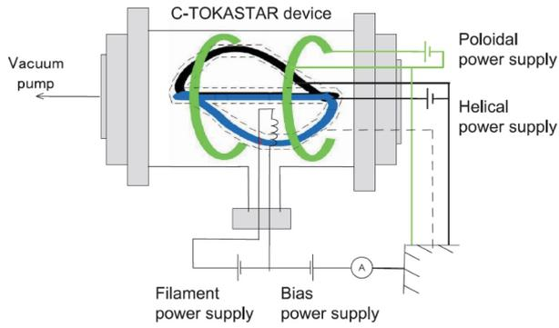
FIG. 3. Experimental setup of the electron-emission impedance method in  $N = 2$  C-TOKASTAR device.
