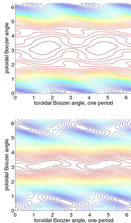
FIG.11. Mod-B contours in the Boozer coordinates near the plasma edge without (upper) and with (lower) plasma current.
