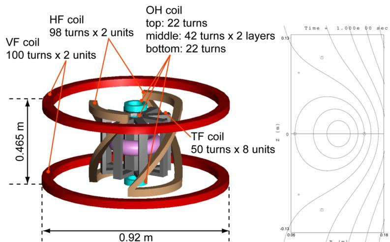
FIG. 5. Coil configuration of TOKASTAR-2 device and magnetic flux surfaces of tokamak operation calculated using TOSCA code.
