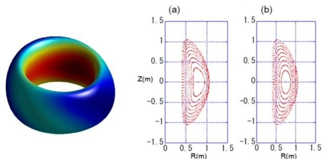
FIG. 2. 3-D plasma configuration (left) of  $N = 2$  C-TOKASTAR and poloidal cross-section of flux surfaces (right) with  $\langle\beta\rangle \sim 4\%$ . (a) current-free equilibrium, (b) flux-conserving  $\langle\beta\rangle \sim 8\%$  equilibrium with plasma current.
