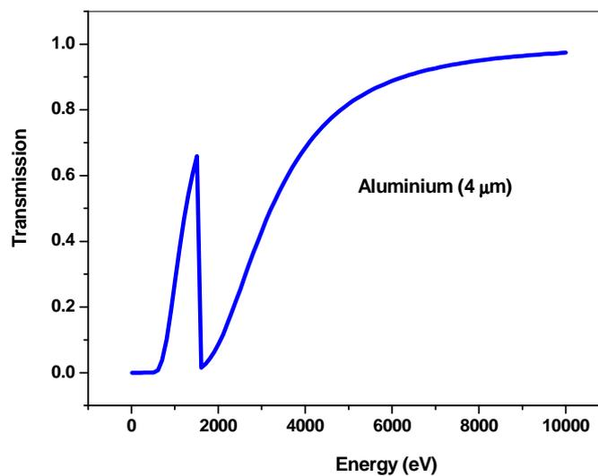
FIG. 7 Transmission curve of aluminum filters ( $4\ \mu\text{m}$ ) used.
