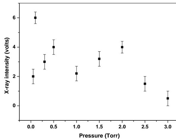
FIG. 8 The variation of the X-ray emission versus helium filling pressure within 0.05-3 torr pressure range
