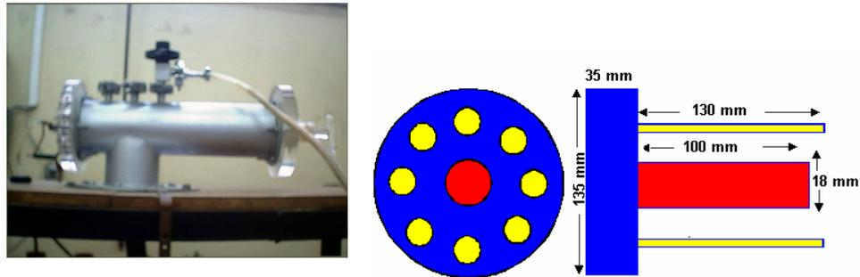
*FIG. 1.* Photograph of plasma focus head and schematic diagram of the construction details of plasma focus electrodes set-up. Right part shows the horizontal cross-section, while the left part shows the vertical cross-section.
