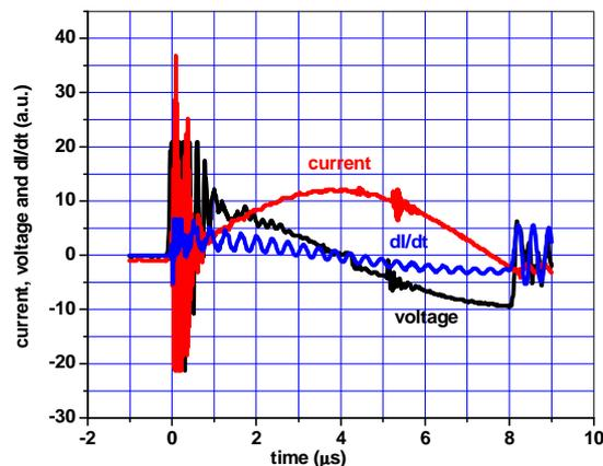
FIG. 3 Discharge current (red), voltage (black) and current dervative (blue) signals from the plasma device.
