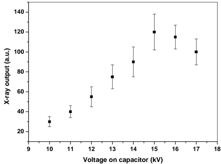
FIG. 6 The relative X-ray output from a dense plasma focus is plotted versus the voltage of the capacitor bank.
