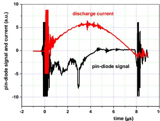
FIG. 5. Oscilloscope of a typical x-ray signal using PIN detector (black) and Rogowski coil signal (red) at 0.1 torr of helium
