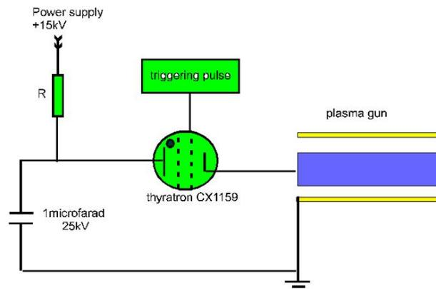
*FIG. 2* The circuit diagram of trigger pulse
