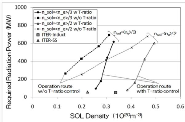
FIG.5 Radiation power required for divertor heat load less than  $10\text{MW/m}^2$  is delineated along the operation route with or without T-ratio control. Two cases of SOL density condition ( $n_{\text{sol}} = \langle n_e \rangle / 3$  and  $n_{\text{sol}} = \langle n_e \rangle / 2$ ) are shown.
