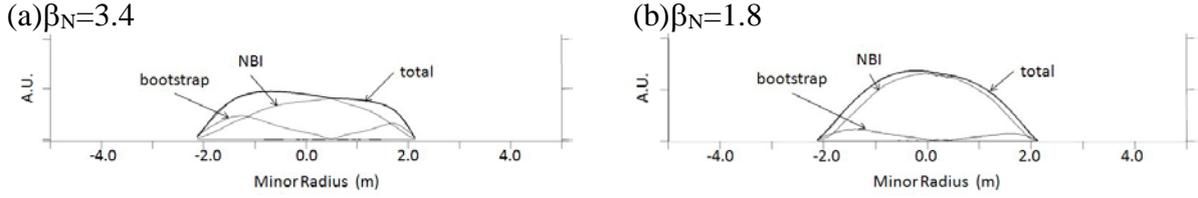
FIG.4 Current profiles for (a)  $\beta_N=3.4$  case and (b)  $\beta_N=1.8$  case for T-ratio  $fn_T=30\%$
