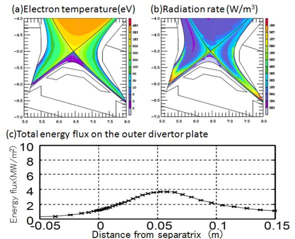
FIG.6 Results of SOLPS, (a) temperature, (b) radiation rate, and (c) energy flux on the outer divertor plate
