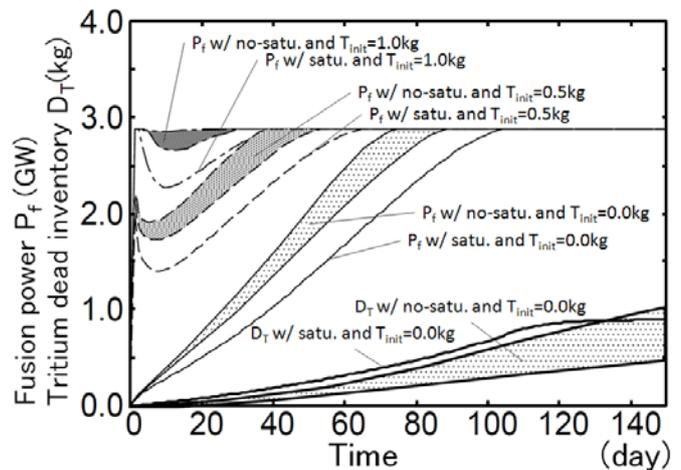
FIG.7 Time evolution of fusion power( $P_f$ ) for  $T_{\text{init}}=0.0, 0.5, 1.0\text{kg}$  and dead inventory in the plasma region( $D_{\text{T}}$ ) for  $T_{\text{init}}=0.0\text{kg}$ . The shaded zones corresponding to the no-saturation case and the lines to the saturation case.
