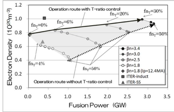
FIG.3 Operational space with T-ratio control for Demo-CREST and ITER operation points
