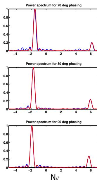
FIG. 5. Comparison of parallel spectra of launched power. The spectra calculated based on the phase measurements of the RF probes (blue) and ideal spectra based on the phase setting of the waveguide (red)
