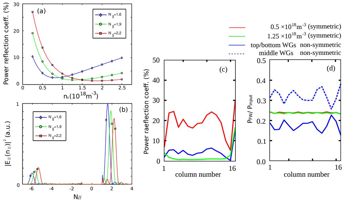
FIG. 3. (Left) the power reflection coefficient (%) as the function of  $n_0$ , and the launched spectrum (b), when the plasma load is uniform in the poloidal direction ( $n_0 = 1.25 \times 10^{18} \text{m}^{-3}$ ). (Right) the impact of poloidal asymmetry of the density in front of the grill. The power reflection coefficient (%) at the input port of four way splitter on each column (c), and the normalized forward power on rows (d). ( $N_{\parallel} = 1.9$ )
