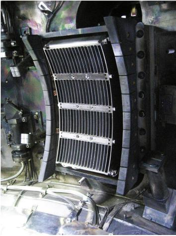
*FIG. 2. Plasma side view of the LH2 launcher installed on Alcator C-Mod. The 16-by-4 active waveguides, 8 passive waveguides, and the surrounding launcher protection limiter can be seen.*
