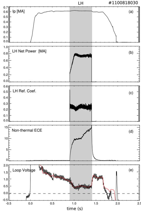
FIG. 6. Temporal evolution of (a) the plasma current, (b) the LH power, (c) the LH coefficient evaluated at the front side of the launcher, (d) non-thermal ECE emission, and (e) loop voltage measured at a flux loop and at the plasma surface (red).
