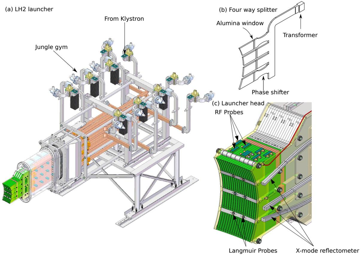
FIG. 1. Schematics of (a) the LH2 launcher, (b) four way splitter, and (c) the coupler waveguide assembly and dedicated diagnostics.
