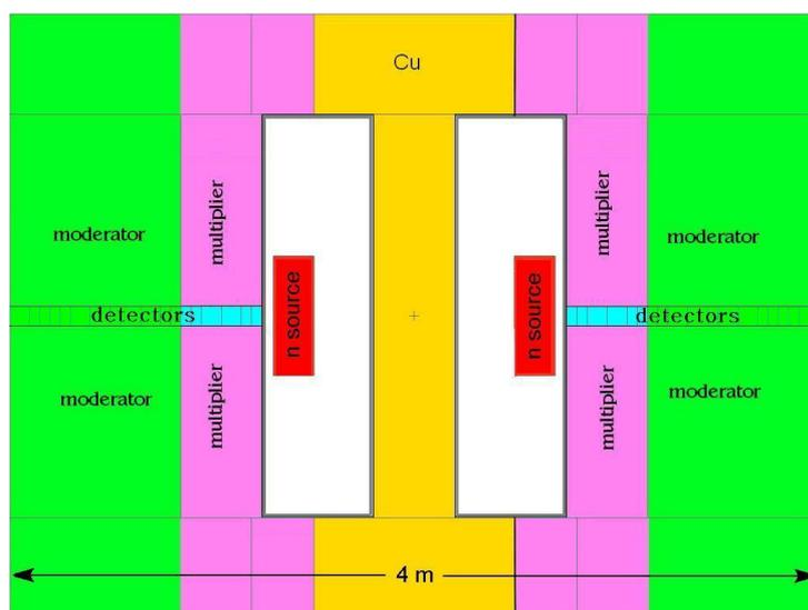
*Fig. 6. Model configuration used in the FNS-ST neutronics analysis.*
