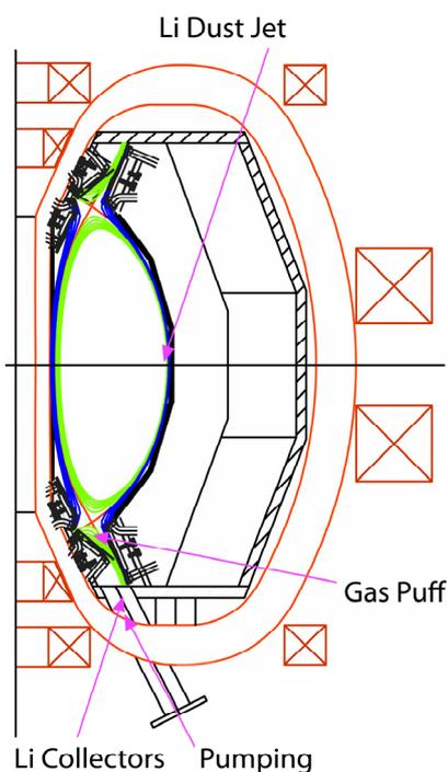
Fig. 5. Schematic of the FNS-ST divertor.
