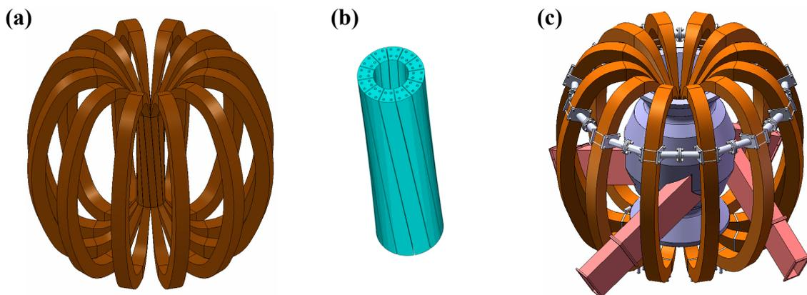
*Fig. 1. The toroidal magnetic system: Cu alloy, 20 tons, 80 m length, 250 kA current, 46.8 V, 11.7 MW, 1.35 T at  $R = 0.47$  m,  $T_{max} = 132^\circ \text{C}$  (a) with twisted central pole (b). Assemblage of the vacuum chamber is fulfilled inside the TF magnet (c).*
