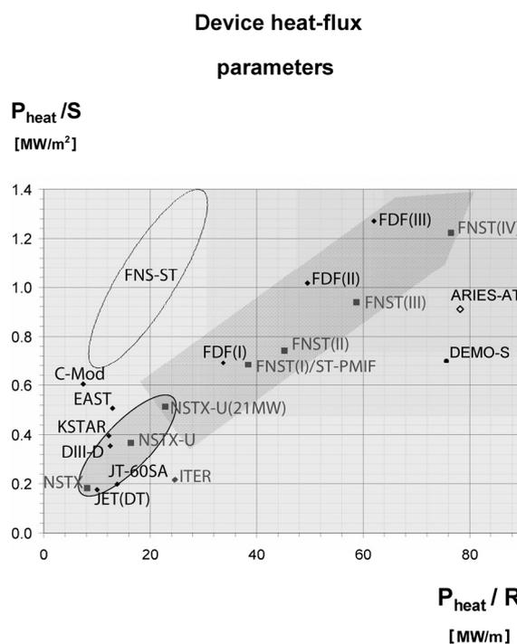
Fig. 4. Wall and divertor power loads of FNS-ST. Operation limits of FNS-ST are placed at the plot illustrating US fusion development program [7] and Russian DEMO-S.
