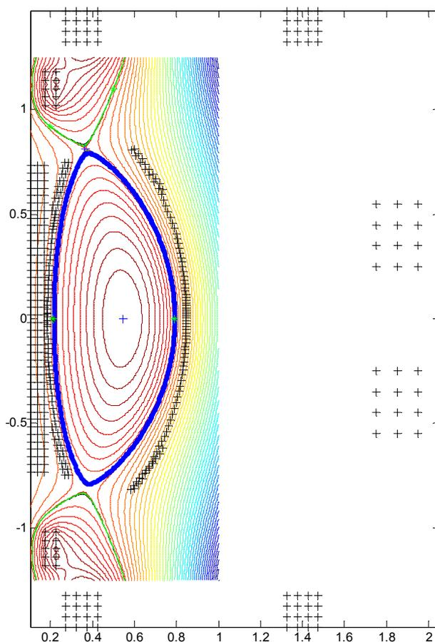
Fig. 3. Equilibrium magnetic configuration at  $I=3 \text{ MA}$  used for evaluations of the maximal values of magnetic coils power consumption and VDE growth rates.
