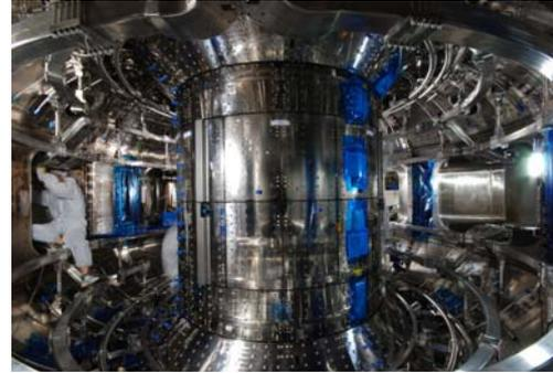
*FIG. 3. Back-plate of divertor after installation*
