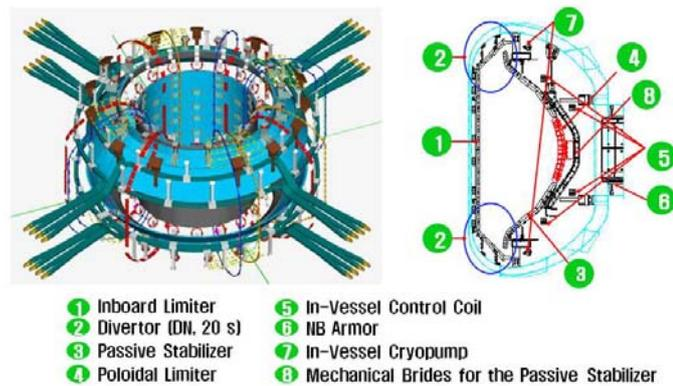
FIG. 1. KSTAR In-vessel components
