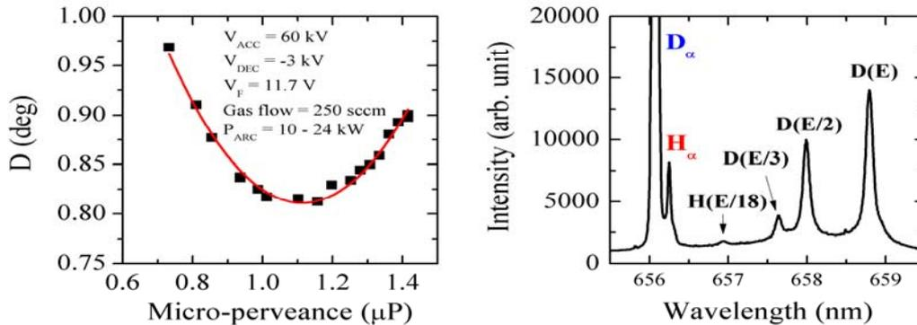
FIG. 12. (Left) beam divergence and micro perveance, and (right) a Doppler shifted spectrum in the beam extraction experiments.
