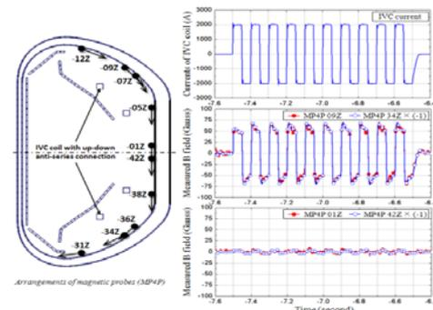
FIG. 8. Result of magnetic field analysis vs. current charging on the IVC coil
