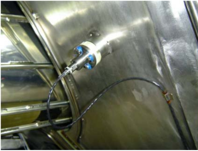
FIG. 10. AE sensor on the TF coil structure
