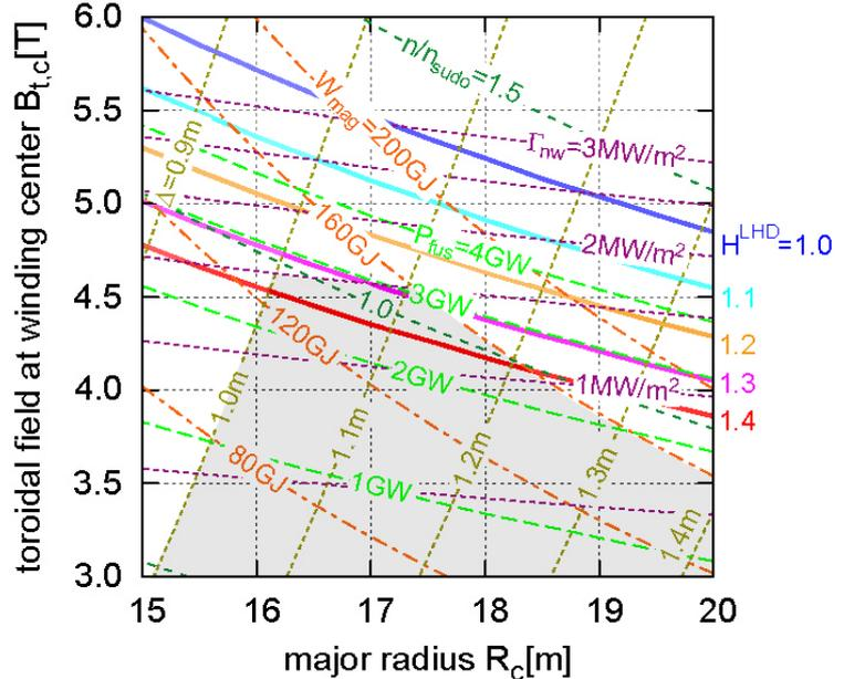
FIG. 6. Contour lines of the design parameters for the case of  $\gamma=1.15$  and  $\langle\beta\rangle = 5.5\%$ . The shadowed region corresponds to the design window satisfies all engineering and physics constraints.
