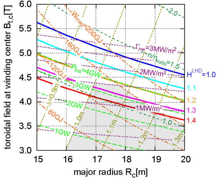
FIG. 5. Contour lines of the design parameters for the case of  $\gamma=1.20$  and  $\langle\beta\rangle = 5.5\%$ . The shadowed region corresponds to the design window satisfies all engineering and physics constraints.
