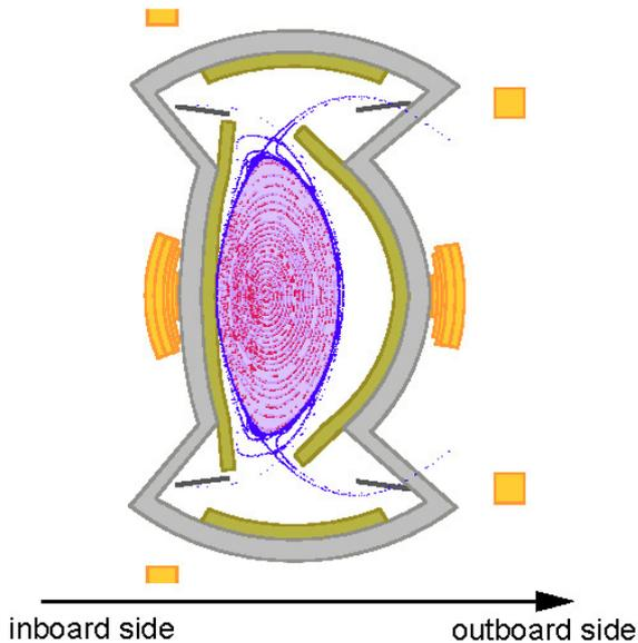
FIG. 1. Cross-sectional view of magnetic surfaces, blankets, shields and coils of the LHD-type heliotron reactor on the cross-section with the minimum blanket space at inboard side.
