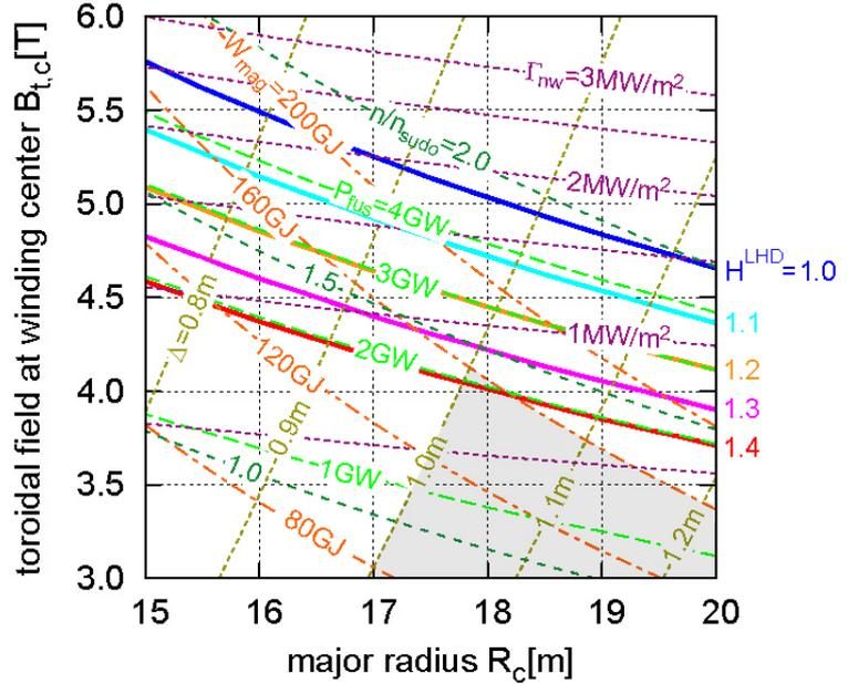
FIG. 7. Contour lines of the design parameters for the case of  $\gamma=1.25$  and  $\langle \beta \rangle = 4.5\%$ . The shadowed region corresponds to the design window satisfies all engineering and physics constraints.
