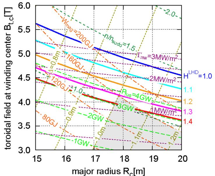
FIG. 4. Contour lines of the design parameters for the case of  $\gamma=1.25$  and  $\langle \beta \rangle = 5.5\%$ . The shadowed region corresponds to the design window satisfies all engineering and physics constraints.
