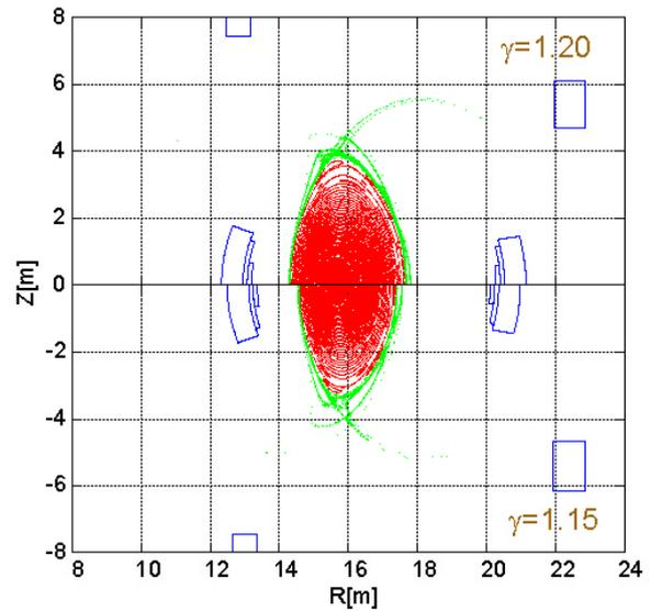
FIG. 2. Comparison of the shapes of the external coils and the magnetic surfaces with the helical pitch parameter  $\gamma$  of 1.20 (upper) and 1.15 (lower).
