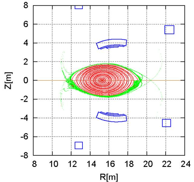
FIG. 3. Comparison of the magnetic surface structure with the original (lower) and the optimized (upper) positions of the vertical field coils.
