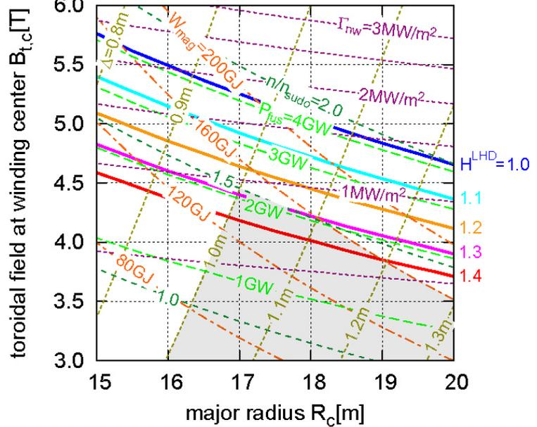
FIG. 8. Contour lines of the design parameters for the case of  $\gamma=1.20$  and  $\langle \beta \rangle = 4.5\%$ . The shadowed region corresponds to the design window satisfies all engineering and physics constraints.
