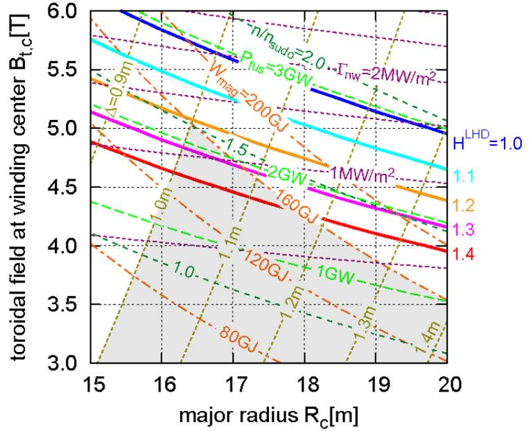
FIG. 9. Contour lines of the design parameters for the case of  $\gamma=1.15$  and  $\langle \beta \rangle = 4.5\%$ . The shadowed region corresponds to the design window satisfies all engineering and physics constraints.
