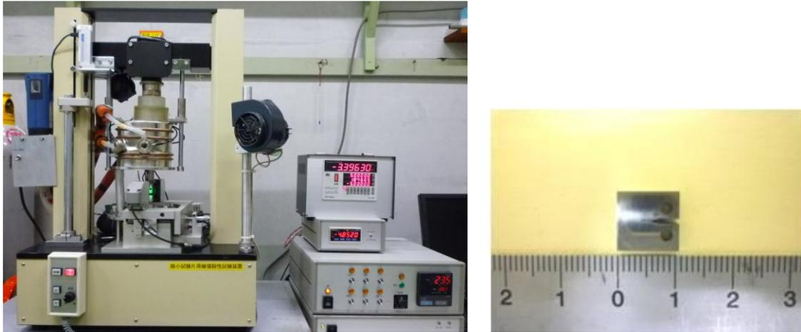
FIG. 4. Developed test machine (Left side) of fracture toughness for small size specimen (Light side).
