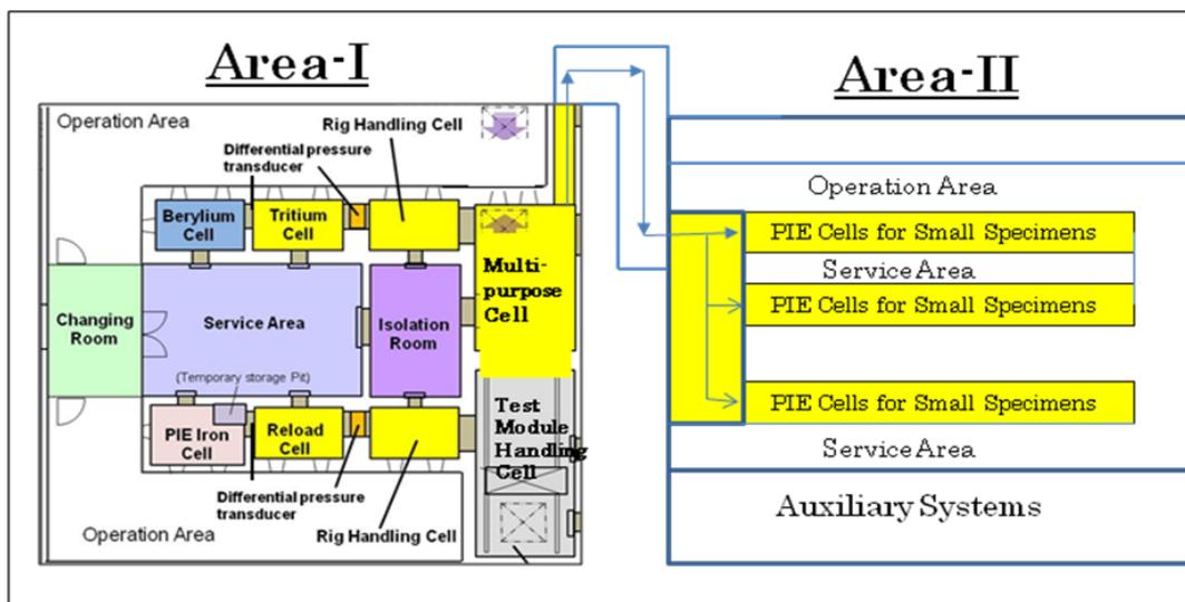
FIG. 1. 2-D image of hot cells for PIE facility. The irradiation rigs are handled in Area-I and PIE for small specimens is mainly performed in Area-II.
