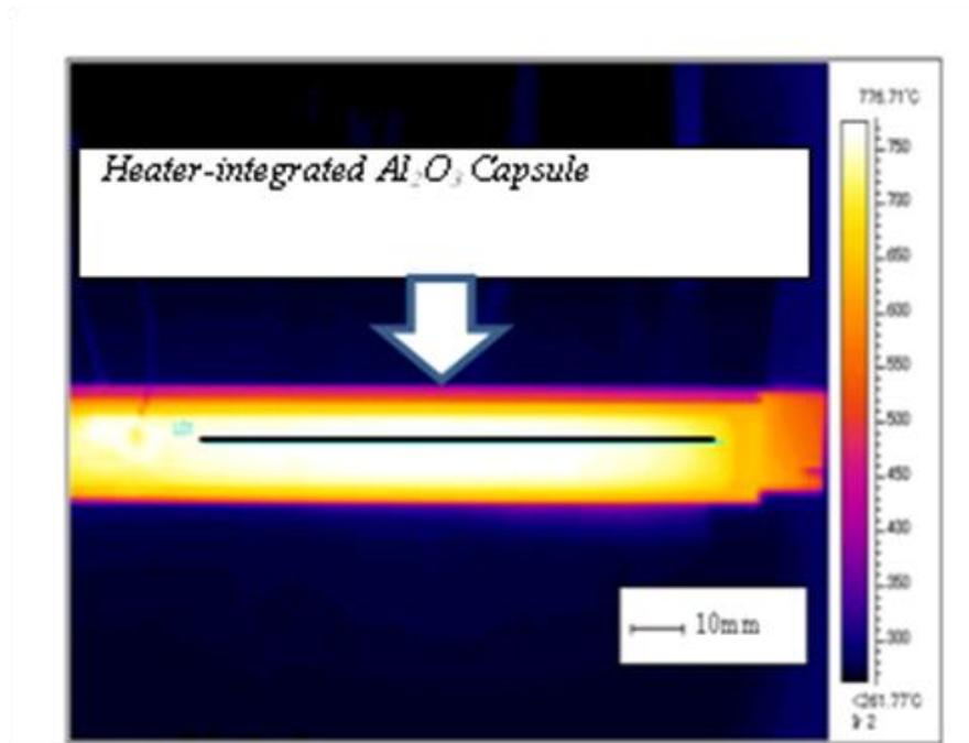
FIG. 3. Uniform temperature distribution of heater-integrated  $\text{Al}_2\text{O}_3$  capsule can be seen at  $760^\circ\text{C}$ . The deviation of temperature is within about  $5^\circ\text{C}$  as shown in the black line.
