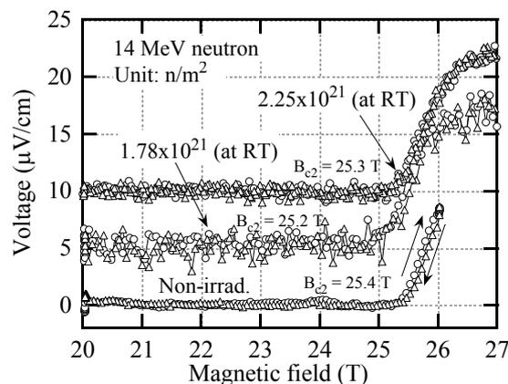
FIG.3. Results of  $B_{C2}$  measurements of  $Nb_3Sn$  strand under 100 mA.
