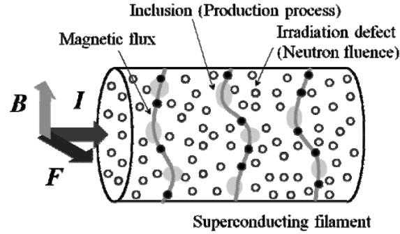
FIG.7. Schematic drawing of pinning sites in irradiated  $Nb_3Sn$  filament.
