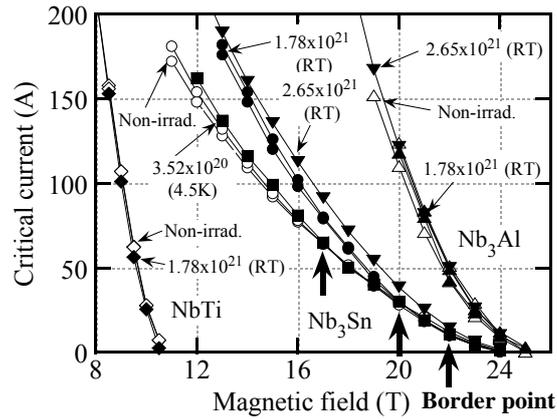
FIG.2. Change in  $I_C$  of  $Nb_3Sn$  strand by neutron irradiation.
