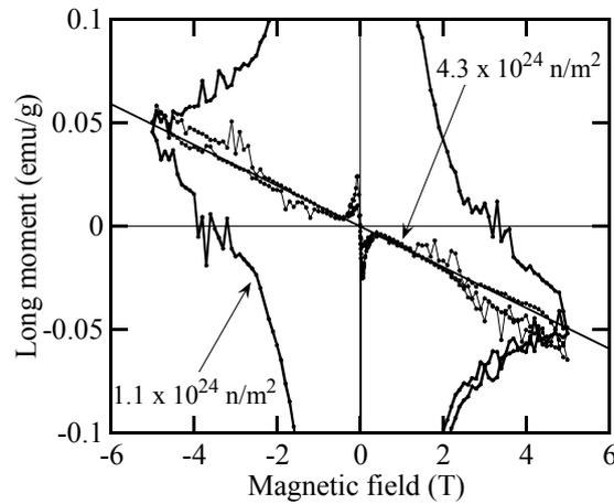
FIG.9. Magnetization diagrams of irradiated  $Nb_3Sn$  strands to  $1.1$  and  $4.3 \times 10^{24}$   $n/m^2$ .
