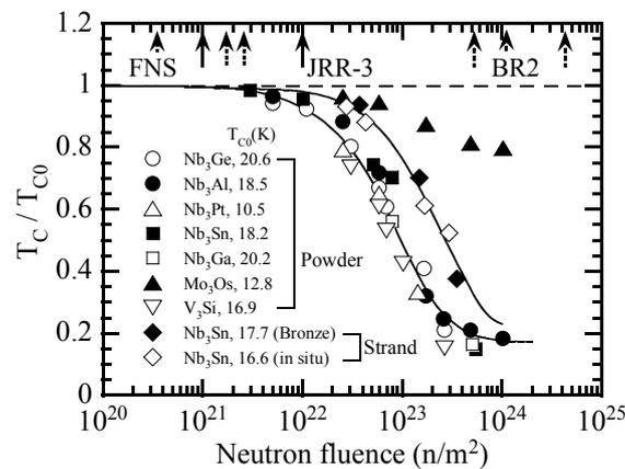
FIG.6.  $T_C/T_{C0}$  of A-15 powders and  $Nb_3Sn$  strands against neutron fluence ( $> 0.1$  MeV) [3,6].
