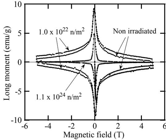
FIG.8. Magnetization of non-irradiated and irradiated  $Nb_3Sn$  strands.
