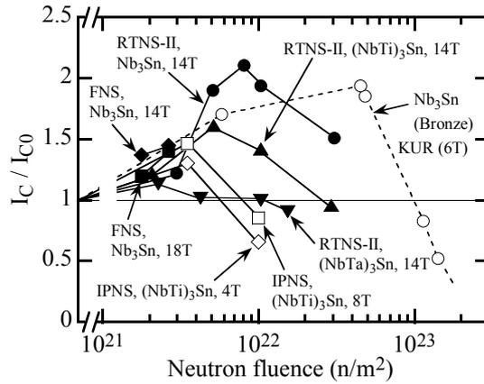
FIG.4.  $I_C/I_{C0}$  of  $Nb_3Sn$  strand against neutron fluence ( $> 0.1$  MeV) [3-5].
