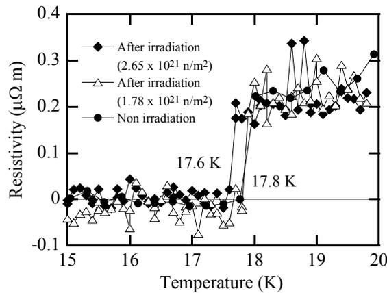
FIG.5. Results of  $T_C$  measurement of  $Nb_3Sn$  strand.
