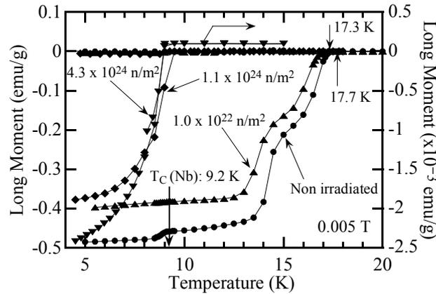
FIG.10.  $T_C$  measurement results of irradiated  $Nb_3Sn$  strand by SQUID.
