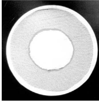
FIG.1. Cross section of  $Nb_3Sn$  strand used.
