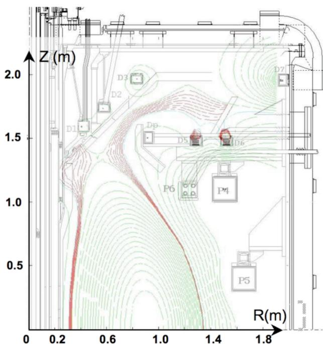
Fig. 2 Super-X engineering design for MAST-upgrade
