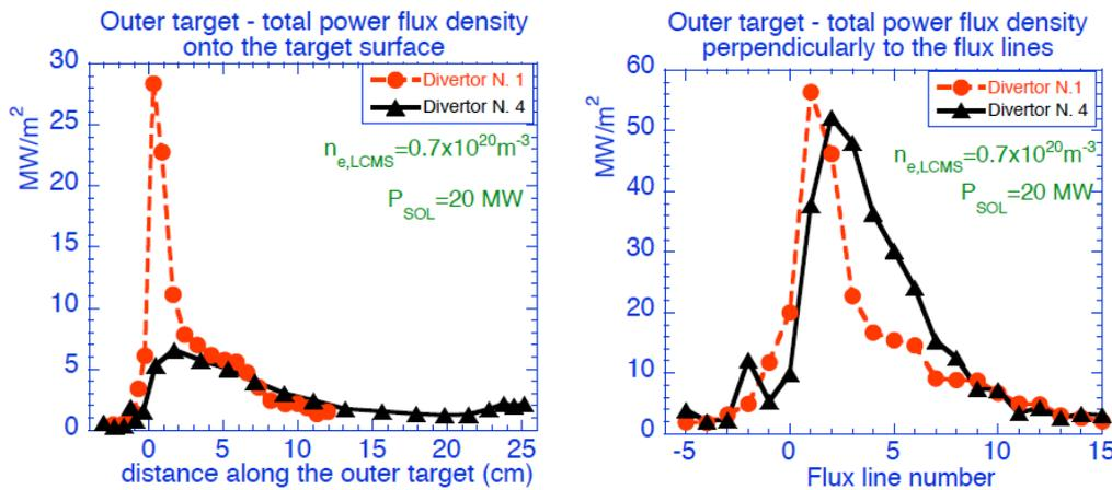
Fig. 4: a) Total Power Load on the outer for divertor shape 1 (strike point angle  $\sim 30^\circ$ ) and divertor shape 4 (strike point angle  $\sim 10^\circ$ ); b) Total power flowing along the tubes flux for the two cases of a).
