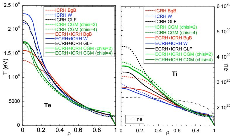
Fig. 2: Ion and electron temperature and density profiles shown for the case of ICRH + ECRH (full line) and full ICRH (dotted line). Red lines are for old BgB, blue for Weiland, black for GLF23 and green for CGM. The assigned density profile is shown with dashed line.
