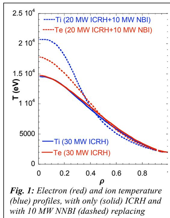
**Fig. 1:** Electron (red) and ion temperature (blue) profiles, with only (solid) ICRH and with 10 MW NNBI (dashed) replacing
