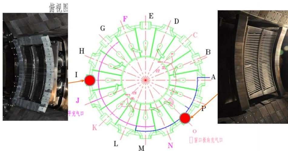
Figure 4 the ICRF Antenna system on EAST
