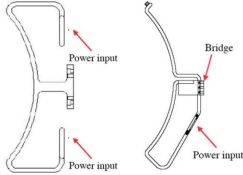
Figure 5 Current strap of 1 port 2-strap antenna (left) and O port 2-strap antenna (right)
