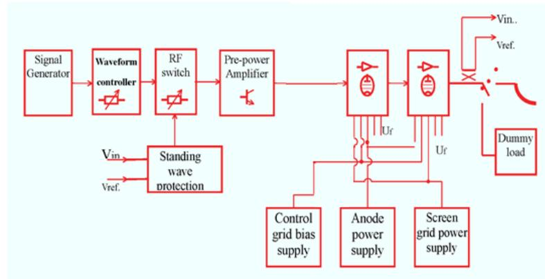
Figure.2 1.5MW RF amplifier
