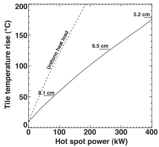
FIG. 8. The ANSYS calculated temperature rise versus the hot spot power with the hot spot foot print taken from SPIRAL (solid line). The dashed line indicates the tile temperature when a uniform heating was assumed.
