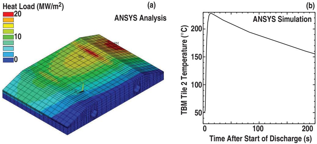
FIG. 7. (a) Initial heat load on the tile using the SPIRAL hot spot and (b) the ANSYS calculated thermocouple response.
