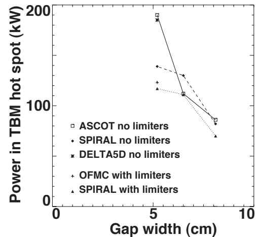
FIG. 6. Hot spot power induced by the TBM fields versus the gap width calculated with various codes.
