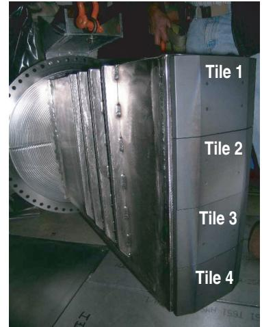
FIG. 1. The four protective carbon tiles on the DIII D TBM mock-up assembly.
