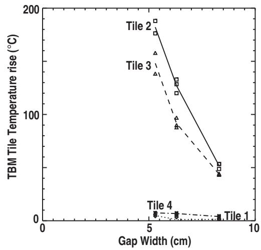
FIG. 4. The measured thermocouple temperature rise at the back of the four tiles for a 1 s long TBM pulse versus the outer gap width. Each symbol is a separate discharge.
