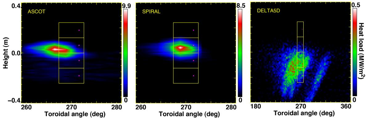
FIG. 5. Heat loads on the first wall near the TBM tiles (yellow outlines) as calculated with the ASCOT, DELTA5D and SPIRAL code for a gap width of 5.2 cm (DIII-D discharge 140156). Note the difference in the color scale. The purple dots indicate the location of the thermocouples at the back of the tiles.
