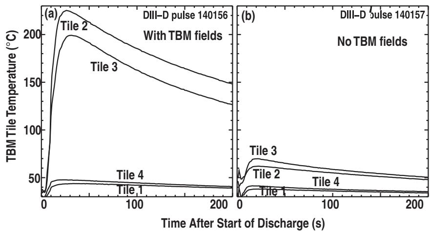
FIG. 2. Tile temperatures measured with the thermocouple at the back of the carbon tiles for two similar DIII-D discharges. In (a) the TBM fields were present while in (b) they were not present.
