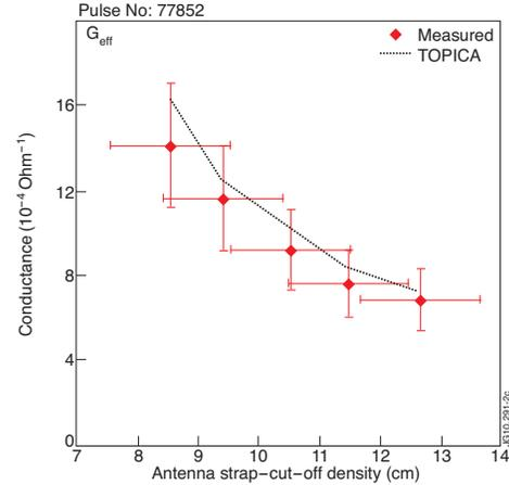
FIG. 7. Comparison of the measured and predicted coupling as represented by  $G_{eff}$  (a proportionality constant between the power coupled and the square of the system voltage)
