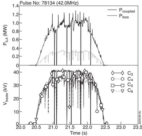
FIG. 6. Pulse JPN 78134. The feeder voltage on strap 1 ( $C_1$ ) is limited at  $\sim 42$  kV limiting the power output of the amplifiers on this pulse with strong ELMs. During the ELMs, when the strap voltage is lower, the power output is raised to the requested value.
