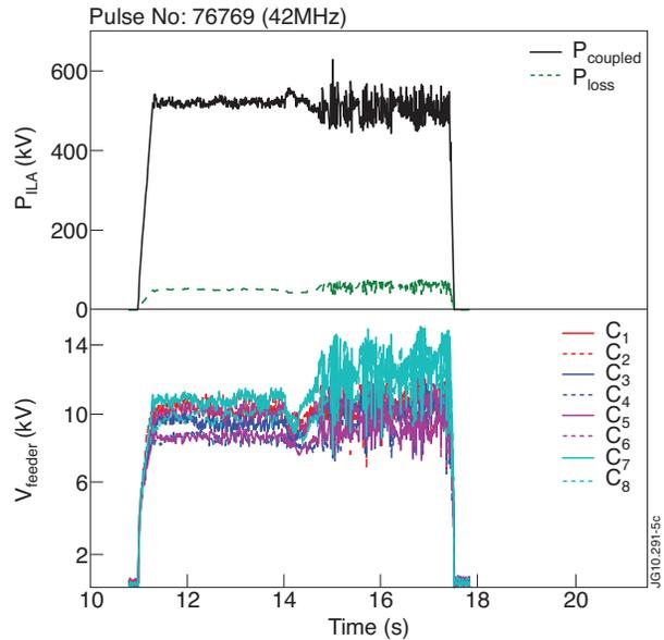
FIG. 8. ILA full array operation during and L-H mode transition (14.5s) and subsequent ELMy H-mode plasma.
