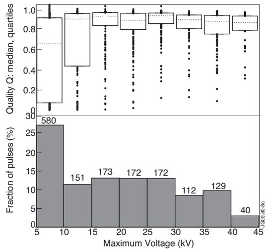
FIG 9. a) quality factor  $Q$  and (b) distribution of the number of pulses vs. antenna voltage. 50% of the pulses lie in the inter quartile's box while 50% of the pulses lie above the dotted median line shown in the box  $Q$  allows discarding the trailing part of pulses that fail due to either power supply issues, amplifiers not restarting correctly after a trip or a lost match and/or insufficient load resilience
