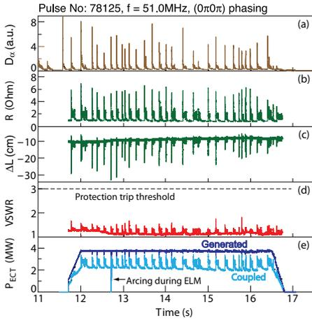
FIG. 3. ECT behavior during big ELMs: (a) mid-plane  $D_{\alpha}$  line emission intensity, (b) antenna strap coupling resistance, (c) antenna strap equivalent length deviation from the vacuum value, (d) VSWR at amplifier output, (e) ICRF power generated and coupled. Plots (b), (c) and (d) are averaged values over the 4 ECT circuits;  $5\mu\text{s}$  RF data sampling.
