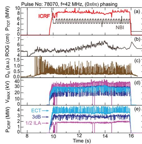
FIG. 4. Example of high power performance of the JET ICRF system during ELMy plasmas: (a) total ICRF and NBI power, (b) mid-plane distance between the separatrix and antenna limiters, (c) mid-plane  $D_{\alpha}$  line emission intensity, (d) maximum voltages on the antenna straps of ILA, ECT and 3dB systems, (e) ICRF coupled power by the ILA, ECT and 3dB system
