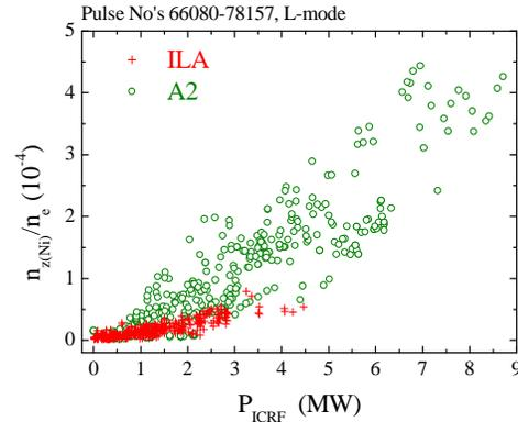
FIG 5. Correlation between Ni concentration ( $r/a \approx 0.5-0.6$ ) obtained with the horizontal VUV spectrometer (KT2) [8] for the ILA (+) and the four A2 (o) antennas as function of the total ICRF power applied.
