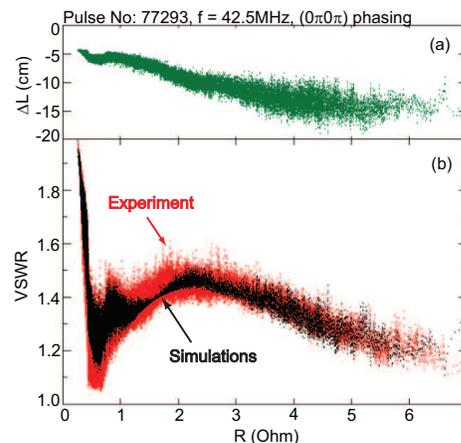
FIG. 2. ECT tolerance to antenna loading perturbations during ELMs: (a) Measured antenna strap equivalent length deviation from the vacuum value (measured) vs. loading variation (b) Measured (red) and simulated (black) VSWR at the amplifier output vs. loading variation; data for one pair of conjugated straps with  $5\mu\text{s}$  sampling over 200 consecutive ELMs.
