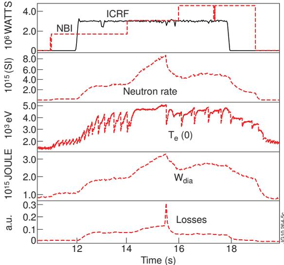
FIG. 5. A typical JET D-plasma discharge 2.2T/ 2.2MA with 3<sup>rd</sup> harmonic ICRH (51MHz) of D beam-ions.
