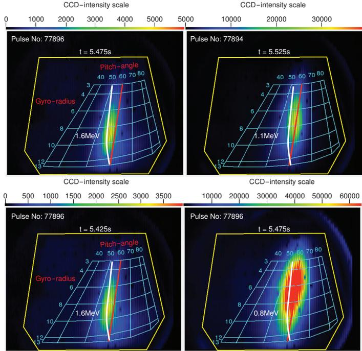
FIG. 4. Footprints of losses detected with SP probe; red line – pitch-angle of the ICRH resonant ions; white line – the trapped-passing boundary on the SP grid.
