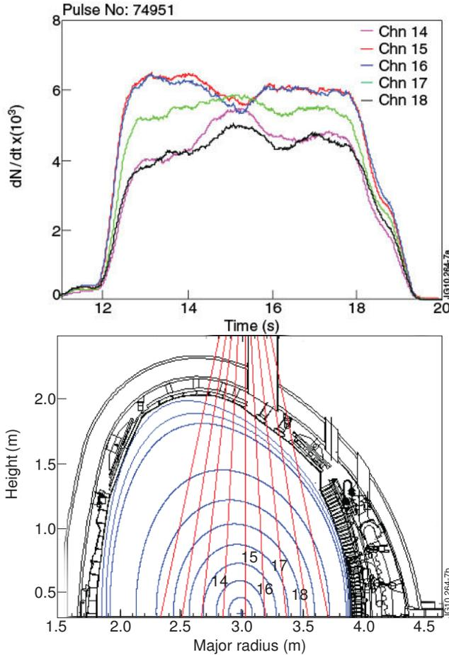
FIG. 7. Top – 3.1-MeV  $\gamma$ -ray intensities vs. time recorded by vertical camera; bottom – the vertical camera lines of sight.
