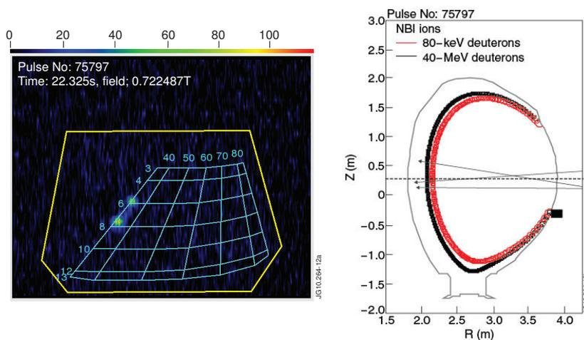
FIG.9. . Footprint of the NBI ion losses; right – orbit of injected D-ions calculated backward in time; arrows show the trajectories of NBI deuterons injected with normal PINI's.
