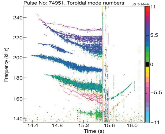
FIG. 6. Magnetic spectrogram showing toroidal mode numbers of TAE and tornado modes before monster sawtooth crash in JPN 74951.
