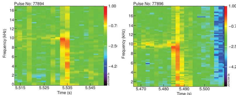
FIG. 2. Magnetic spectrograms showing  $m=2/n=1$  mode in #77894 and #77896.
