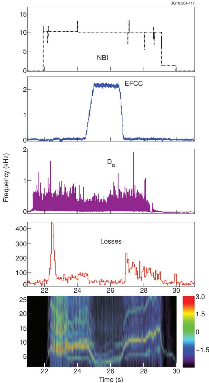
FIG.8. Waveforms and magnetic spectrogram (frequency, kHz vs time) showing 3/2 NTM mode evolution during EFCC (24.5 s– 26.8 s) in the discharge #75797 at  $B_T = 1.0\text{T}$ ,  $I_p = 0.8\text{MA}$  and  $I_{EFCC} = 2.2\text{kA}$ ; integral NBI losses (a.u.) were measured with SP.
