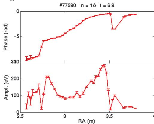
Fig. 12. Phase and amplitude profiles along the major radius on the ECE sightline during the tearing-like stage of the continuous mode, with a clear  $\pi$ -jump of phase and a dip of amplitude on the LFS
