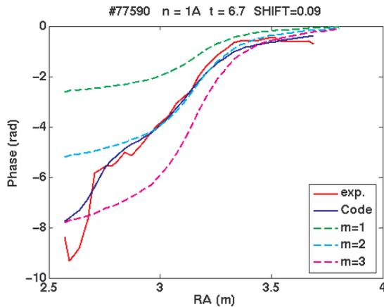
Fig. 13. Measured (red) and calculated (blue) phase profiles along the ECE sightline. Dashed lines show profiles for pure poloidal components.
