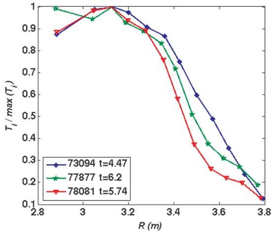
Fig. 8. Normalised ion temperature profiles at  $q_{\min} \approx 1.5$ . Discharge 73094 develops the continuous mode at  $\beta_N = 3.3$ ; 77877 shows mild bursting modes and then the continuous mode at  $\beta_N = 2.6$ ; 78081 has a disruptive bursting mode at  $\beta_N = 2.35$ .
