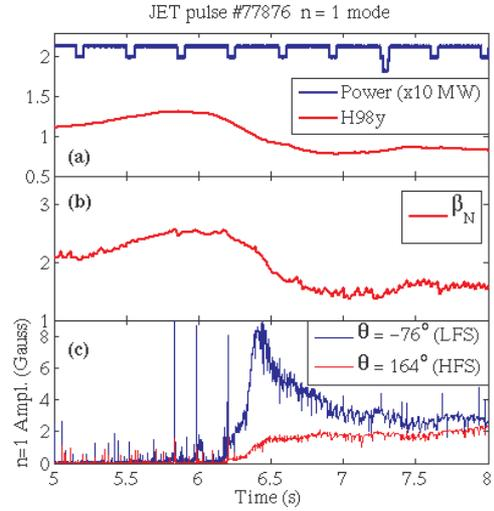
Fig. 2. a) Power and confinement factor waveforms. b) Normalized beta. c)  $n=1$  mode amplitude on LFS (blue) and HFS (red); fishbone-like events appear as spikes. The kink-like stage lasts from  $t = 6.42$  s to  $t = 6.45$  s.
