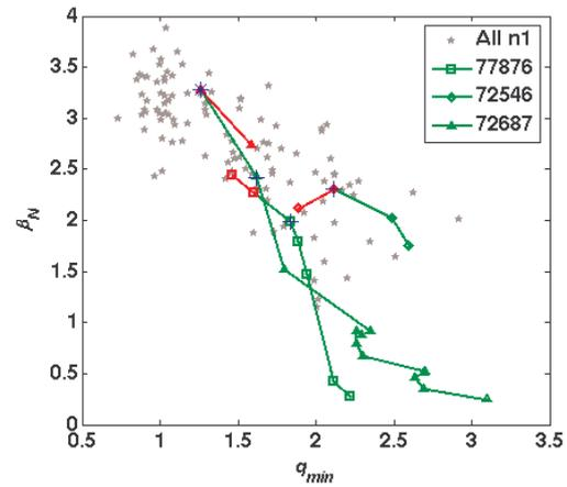
Fig. 4. Trajectories in the operational diagram. Onset of the  $n = 1$  mode occurs at some point of the red segments. Grey stars represent all onsets, like red stars in fig. 3. Crosses and asterisk mark the onset of no-wall and with-wall ideal instability conditions from the MISHKA code.
