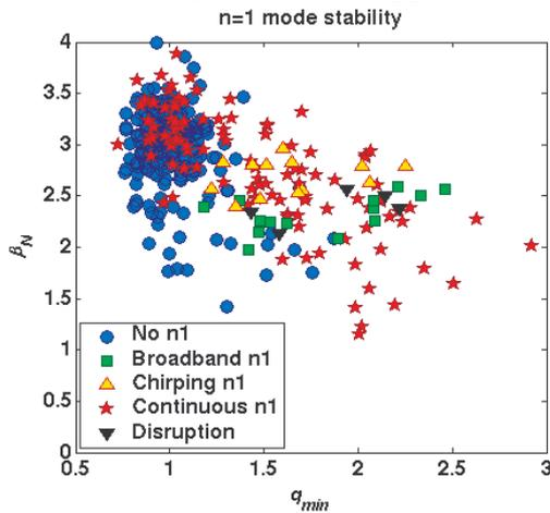
Fig. 3. Operational stability diagram. Blue dots and green squares respectively indicate maximum  $\beta_N$  in discharges without  $n = 1$  modes and with broadband activity only. Yellow triangles and red stars show  $\beta_N$  values at the onset of bursting and continuous  $n = 1$  modes respectively. Black triangles indicate disruptions.
