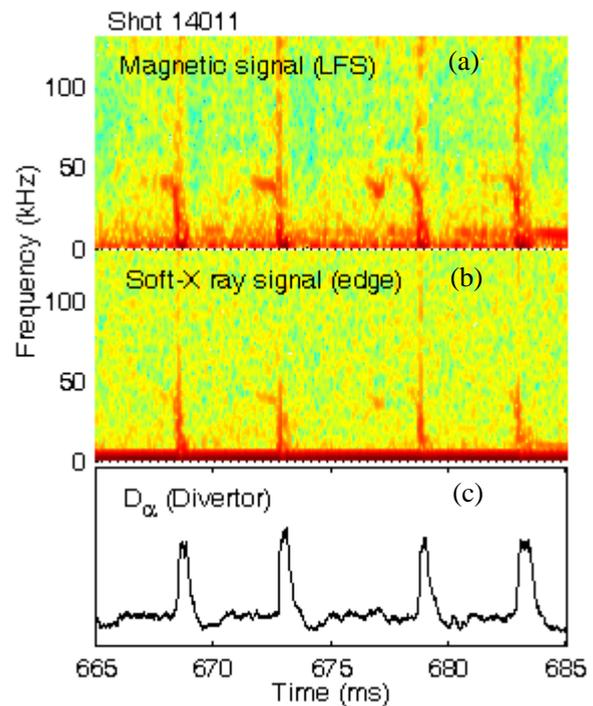
FIG.5. The Spectrogram of the ELM precursors from magnetic probe (LFS) and soft-X ray (edge channel). The divertor  $D_\alpha$  indicates the onset of ELM.
