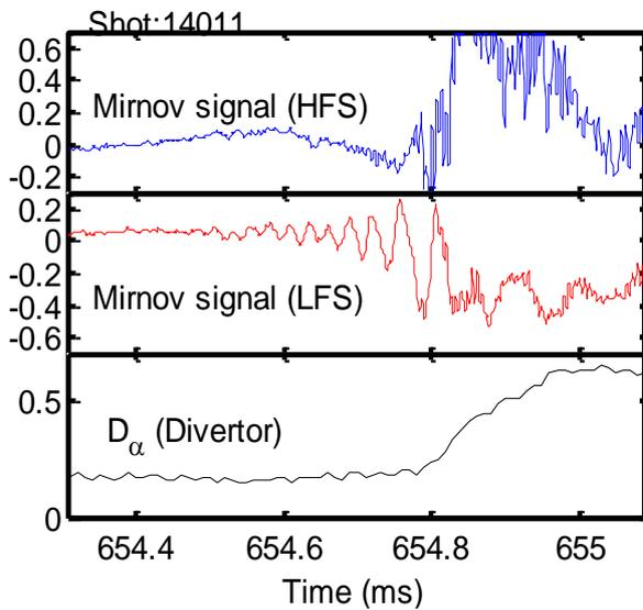
FIG.6. Strong poloidal asymmetry of the precursor is observed by the LFS and HFS Mirnov probes. And the amplitude of the precursor grows rapidly before the ELM crash
