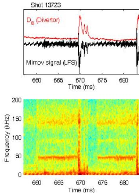
FIG4. Magnetic fluctuations during an ELM
