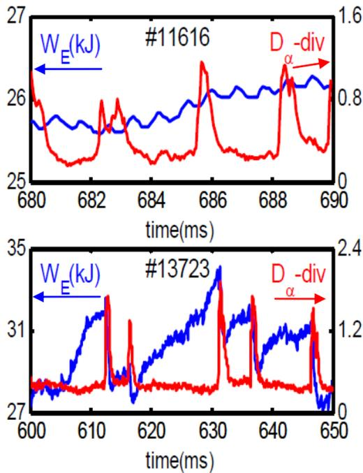
FIG3, energy loss for an ELM
