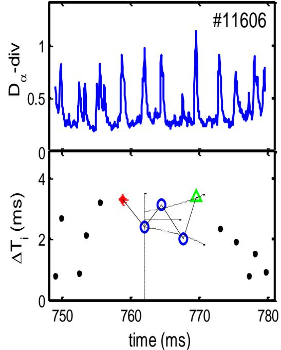
FIG9, top plot is the  $D\alpha$  signal of the ELMs and the bottom is a UPO candidate.
