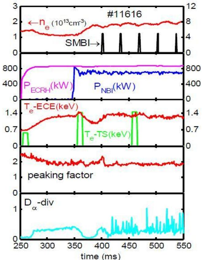
FIG.1. A typical discharge of H-mode with Type-III ELMs in HL-2A.
