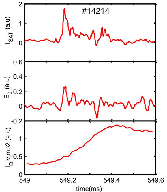
FIG.7. Ion saturation current  $I_{STA}$  and poloidal electric field  $E_\theta$  in a filament
