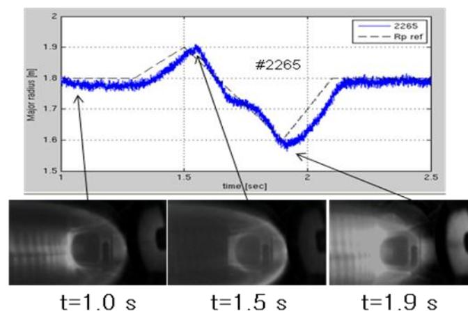
**Fig. 3. Plasma major radius (Rp) controls matching with the fast-frame CCD camera (380frames/sec) in the circular plasmas.**
