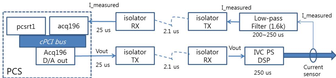
**Fig. 7. Design of the feedback loop of the KSTAR PCS for the IVC PS**
