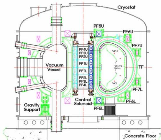
**Fig. 1. Coil & structure geometry of the KSTAR in 2010.**
