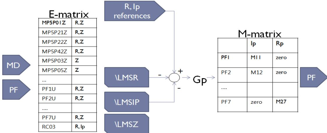
**Fig. 4. Design of the R, Z & Ip feedback loop of the KSTAR PCS: the Estimator matrix (E-matrix) consists of response weights on magnetic probes and PF coils, and multiplication matrix (M-matrix) determines how the PCS responses are distributed on each actuator.**
