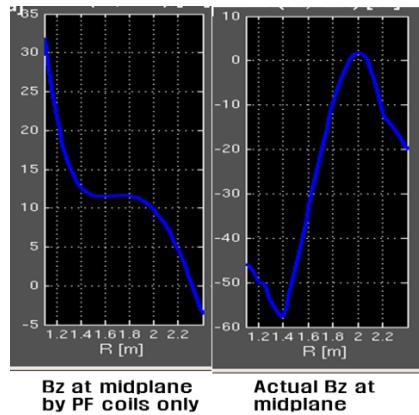
**Fig. 2. Vertical field (Bz) reconstructions produced by PF currents (left) and real measurement (right).**
