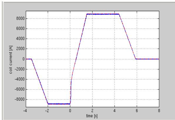
**Fig. 9. Bipolar swing example of the KSTAR PF3U from -9 kA to +9 kA/turn.**
