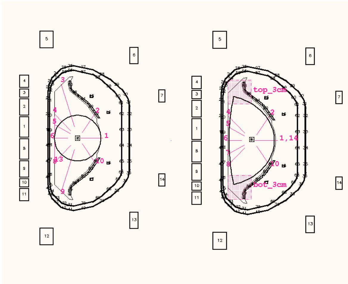
**Fig. 11. Generalized shape editor installed to the KSTAR PCS : definitions of control segments for limited/elongated plasma (left) and up/down symmetric double-null plasma (right).**
