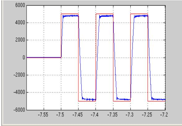
**Fig. 8. Fast swing test of the in-vessel vertical coil (IVC) with +5 kA/turn, 10 Hz.**
