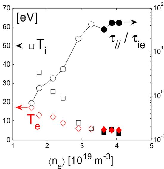
FIG. 4. Ion and electron temperatures measured by Retarding Field Analyser at the LCFS in ohmic density scan in Tore Supra. The ratio of the parallel ion transit time through the SOL to the ion-electron thermalization time evaluated 2-3 cm outside the LCFS indicates the degree of the ion-electron collisional coupling. Full symbols: detached discharges.
