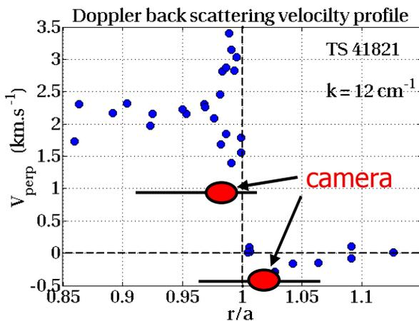
FIG. 2. Poloidal velocity profiles measured by Doppler back scattering with measurements from fast camera images super-imposed (positive velocity is in the electron diamagnetic direction).
