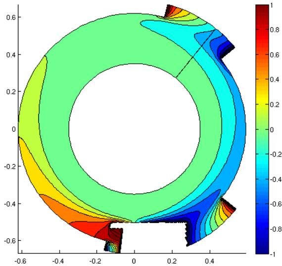
FIG. 5. Poloidal color plot of the parallel velocity (normalized to the sound speed) obtained with the SOLEDGE-2D code in a realistic Tore Supra geometry for poloidally uniform transport coefficients.
