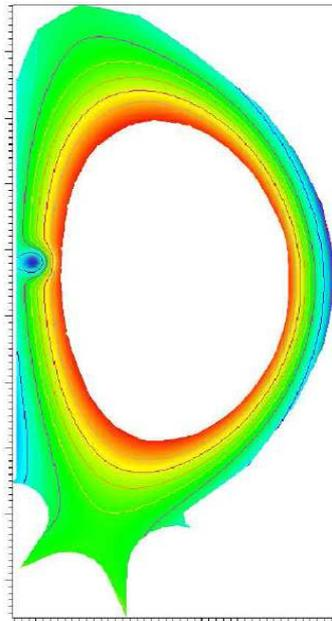
FIG. 10. Colour map of the electron temperature obtained with the ESPOIR code after seeding of a cold radiative spot in the HFS.
