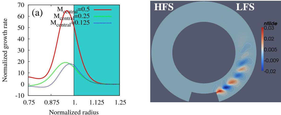
FIG. 9. a) radial profile of the normalized growth rate of the parallel shear flow instability in the most unstable region, i.e. just on the LFS of the floor limiter. Profiles for 3 different core rotations are plotted.  $r=1$  corresponds to the LCFS. b) colour map of the density (equilibrium subtracted) showing the development of the instability at the tip of the limiter on the LFS.
