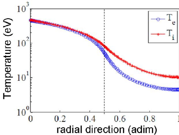
FIG. 7. Poloidally averaged temperature profiles obtained with the SOLEDGE-2D code for a typical Tore-Supra case. The width of the radial domain is 10cm and the last closed flux surface is at  $r=0.5$  (dashed line).
