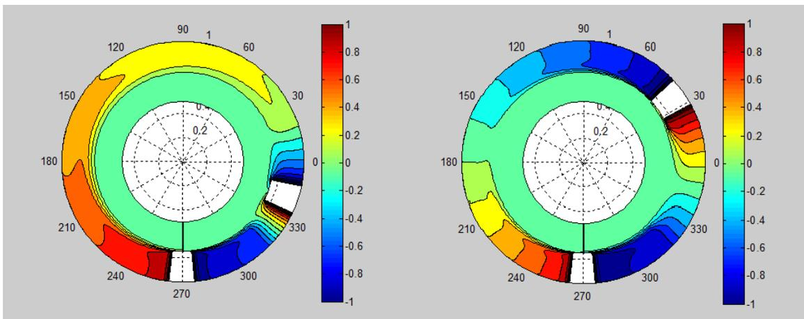
FIG. 6. Poloidal color plot of the parallel velocity (normalized to the sound speed) obtained with the SOLEDGE-2D code for 2 different poloidal positions of the secondary limiter in the LFS, including ballooned transport coefficients in line with experimental findings. Note the flow reversal at the top.
