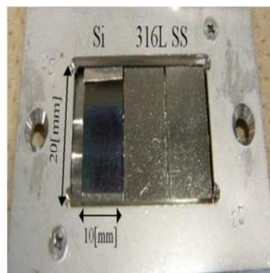
FIG. 4 Material probe holder installed in the 11<sup>th</sup> campaign.
