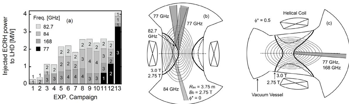
FIG. 1. (a) the history of ECRH port-through power, the injected EC wave beams in (b) the vertically and (c) the horizontally elongated magnetic surface for the magnetic configuration of  $R_{ax} = 3.75$  m,  $B_t = 2.75$  T.
