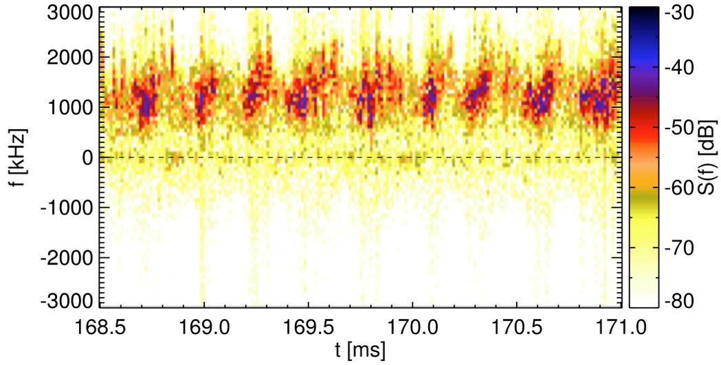
FIG. 3: Spectrogram of the Doppler reflectometer signals measured at  $\rho \approx 0.8$  in the magnetic configuration with  $\nu/2\pi = 1.63$  at the plasma edge. The colour code reflects the density fluctuation level and the frequency of the Doppler peak gives  $E_r$ . A short time interval is displayed in order to follow closely few oscillation cycles.
