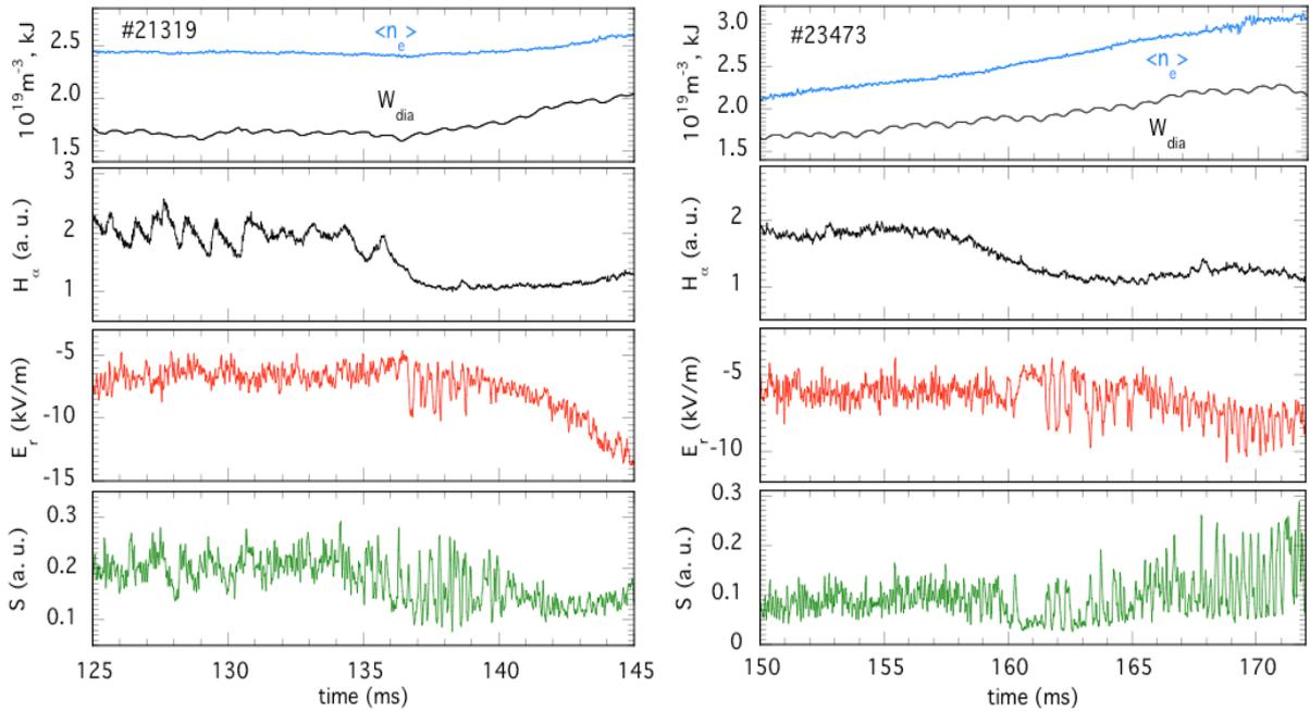
FIG. 1: The time evolution of line-averaged plasma density, plasma energy content,  $H_\alpha$  signal, and  $E_r$  (in red) and density fluctuation level (in green) measured at  $\rho \approx 0.8$  using the Doppler reflectometer, in two magnetic configurations with edge rotational transform in vacuum  $\nu/2\pi = 1.63$  (left) and  $\nu/2\pi = 1.53$  (right).
