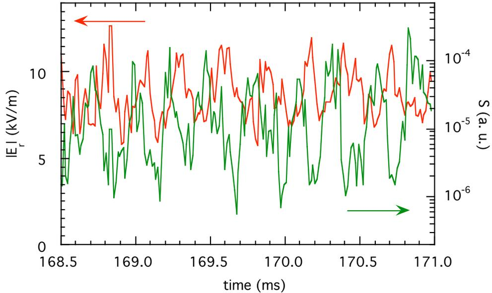
FIG. 4: Time evolution of  $E_r$  (in red) and density fluctuation level (in green) obtained by fitting a Gaussian function to the spectra shown in figure 3.
