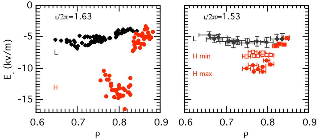
FIG. 2:  $E_r$  radial profiles in L and H-mode plasmas in two magnetic configurations with  $\nu/2\pi$  at the plasma edge 1.63 (left) and 1.53 (right). In the later case (right), the  $E_r$  minima and maxima values measured during the oscillatory phase are represented. No oscillations are seen at the outer radial positions where  $E_r$  remains almost unchanged at the transition.
