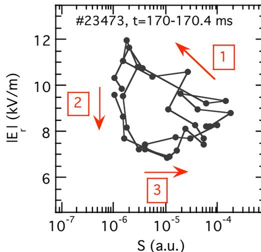
FIG. 5: Relation between  $E_r$  and density fluctuation level. They evolve following closed trajectories in a limit-cycle style. Two of the cycles shown in figure 4 are displayed; the time interval between consecutive points being  $12.8 \mu\text{s}$ .
