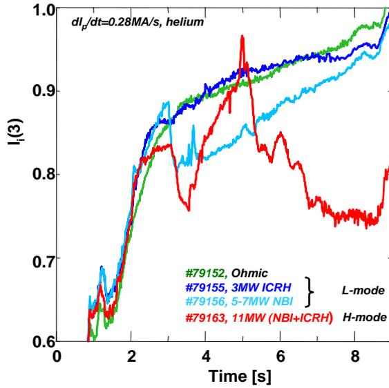
Figure 2: The evolution of the plasma inductance for four helium discharges at various heating levels. Only #79163 makes a transition to H-mode at  $t=3.0s$  and  $t=6.0s$
