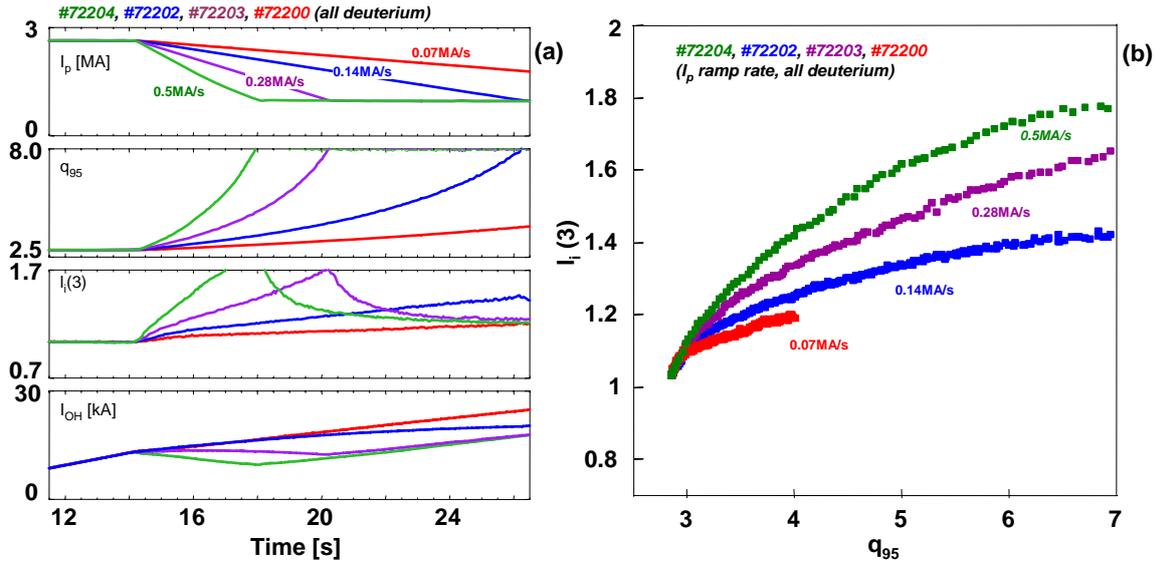
Figure 6: The evolution of four discharges for different current ramp down rates. Figure (a): Plasma current,  $q_{95}$ , plasma inductance and current in the ohmic circuit. (b): Evolution in the  $l_i(3)$ - $q_{95}$  plane.
