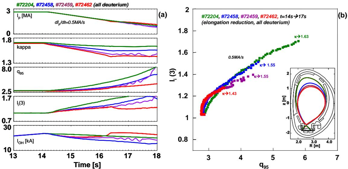
Figure 7: The evolution of four discharges for different elongation reduction during the current ramp down. Figure (a): Plasma current, elongation,  $q_{95}$ , plasma inductance and current in the ohmic circuit. (b): Evolution in the  $l_i(3)$ - $q_{95}$  plane, the inset shows to plasma shape at  $t=16.5$  s
