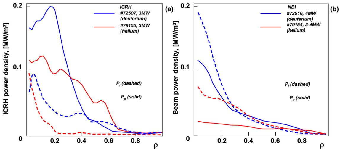
Figure 5: The electron power density profile for two L-mode cases: (a) ICRH heating and (b) NBI. The helium data are compared to deuterium reference cases.
