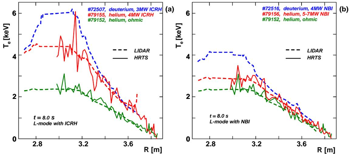
Figure 4: The electron temperature profile for two L-mode cases: (a) ICRH heating and (b) NBI. The helium data are compared to deuterium reference cases and ohmic helium discharges.
