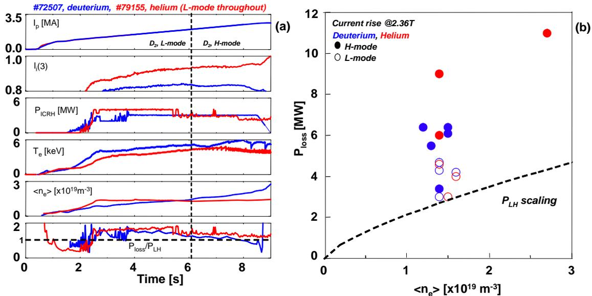
Figure 3: Comparing the H-mode behaviour in deuterium and helium during the current rise phase. Figure (a): Plasma current, plasma inductance, ICRH power, central electron temperature, plasma density and input power normalised to the H-mode threshold scaling for deuterium. (b) Overview of the heating power applied during the current rise phase in deuterium and helium.
