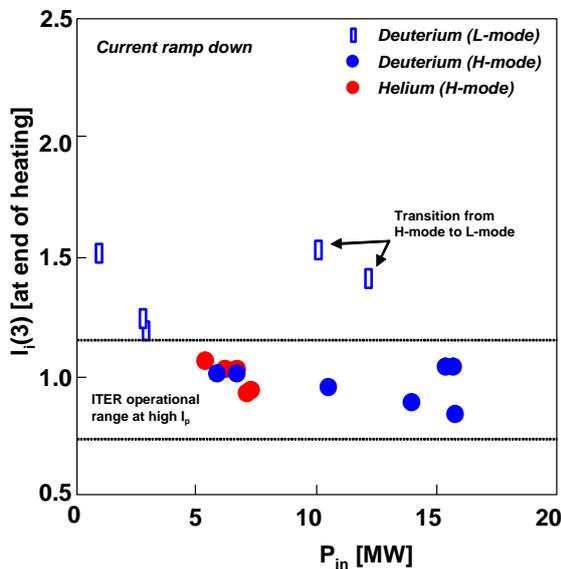
Figure 8: The plasma inductance at the end of the additional heating phase, during the current ramp down, plotted against the applied heating power.
