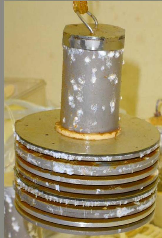
A test rack with coupons, before and after exposure for a year to a spent fuel basin in Serbia.
