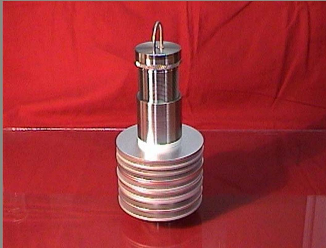
The corrosion test rack with coupons
