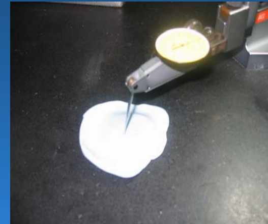
Fig.6. Measurement of swelling height
