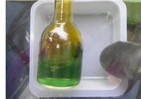
Solution of Am Sample in V-capsule irradiated in JOYO
