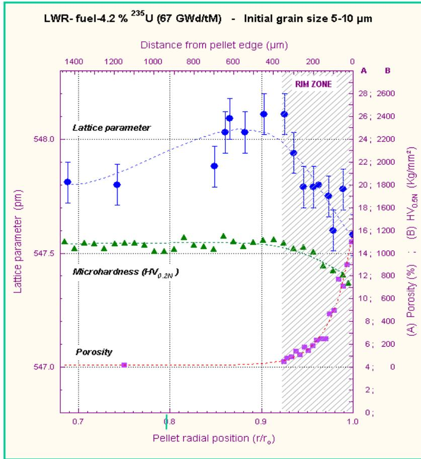
*Microstructure, micro-hardness and lattice parameter variations at the fuel periphery (rim zone)*
