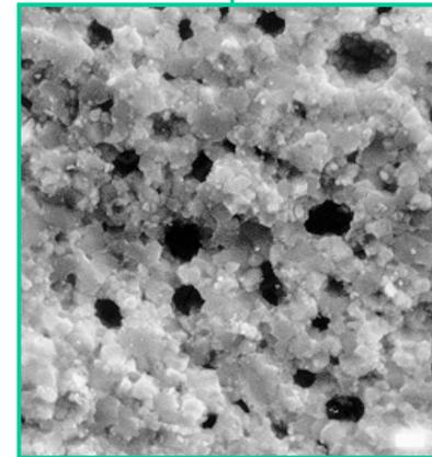
*Microstructure, micro-hardness and lattice parameter variations at the fuel periphery (rim zone)*
