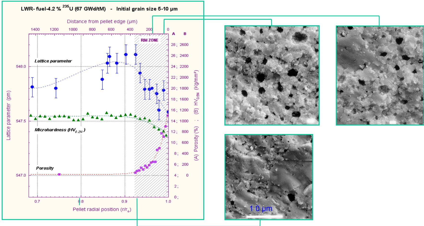
*Microstructure, micro-hardness and lattice parameter variations at the fuel periphery (rim zone)*
