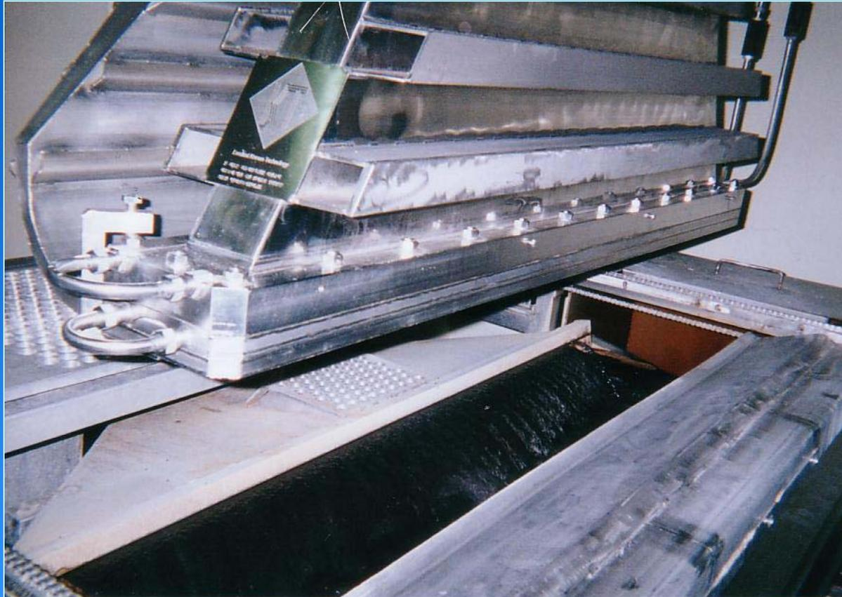
Pilot-scale plant of cleaning waste water from dyeing
