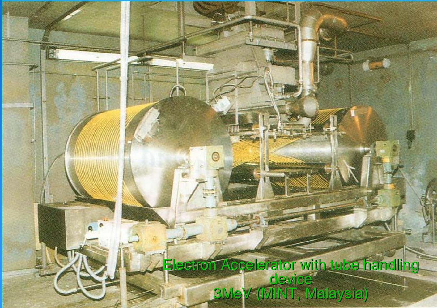
Electron Accelerator with tube handling
