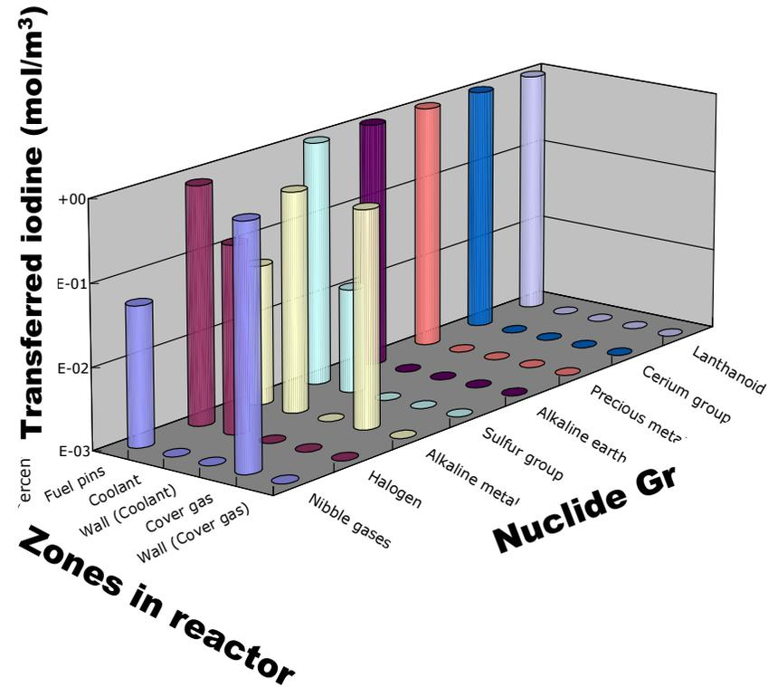
**Distribution of FP nuclides in reactor 100s after cladding failure in PLOHS**
