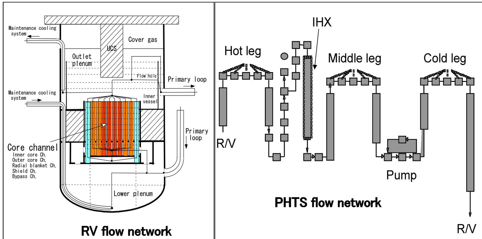
Fig.5 Flow network of the NALAP-II code for RV and PHTS
