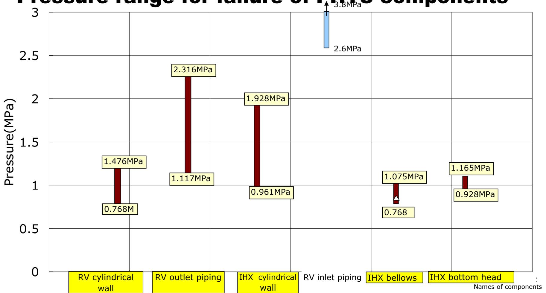
Five locations (RV cylindrical wall, RV outlet piping, IHX cylindrical wall, IHX bellows and IHX bottom head) fail at the pressure between 0.77 to 2.3 MPa).
