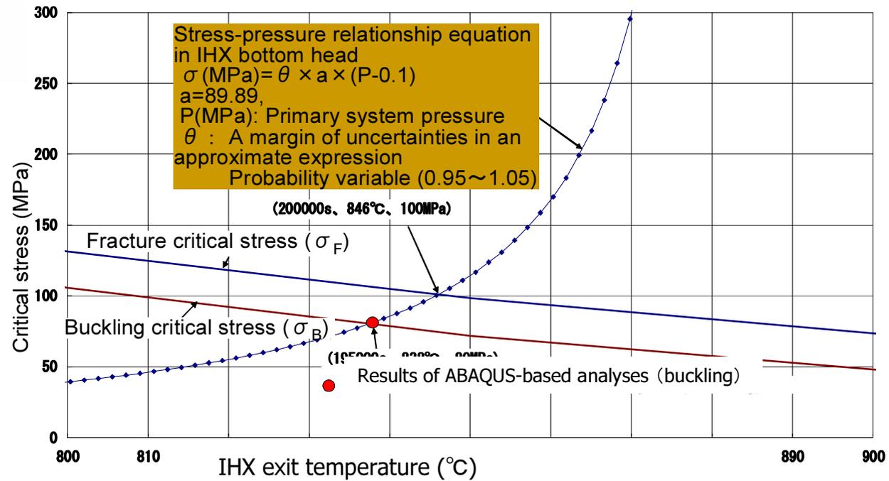
The obtained stress-pressure relation curve encountered with the buckling critical stress line and the fractional critical stress line at one point, respectively. The IHX bottom head is expected to fail at the condition between the two points.
