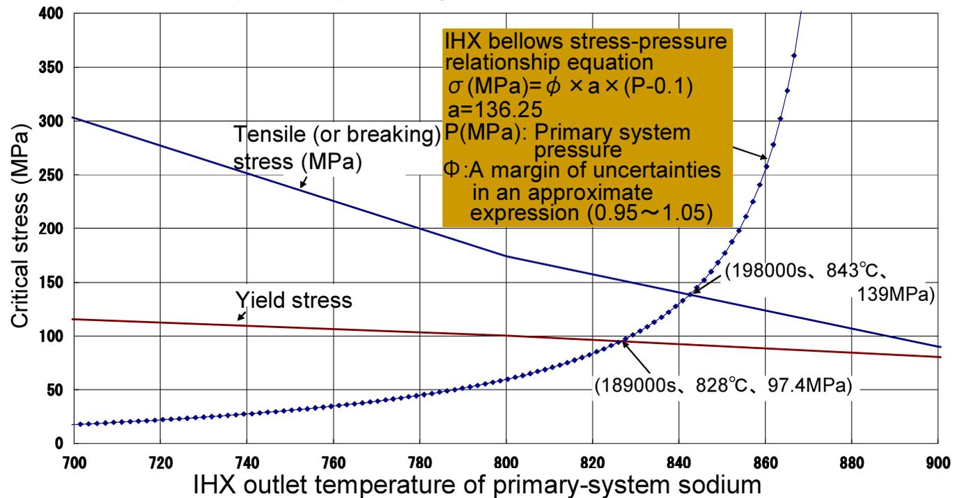
The obtained stress-pressure relation curve encountered with the yield stress line and the tensile stress line at one point, respectively. The IHX bellows is expected to fail at the condition between the two points.
