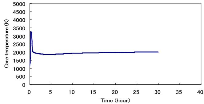
Fig. 7-22(1) Core Temperature (Case 15: PLOHS, Non-CVBP, PL-NSL-H-...)
