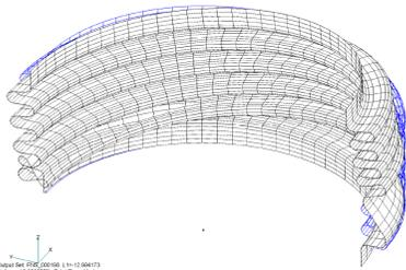
Deformed IHX bellows (Temperature: 750°C; Pressure: 0.388 MPa) (The results of the FINAS 3-d calculation)
