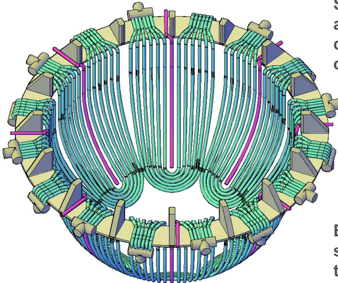
**Reactor Vessel Air Cooling System connected to an inlet air collector and an outlet chimney to promote natural circulation.**
