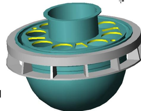
**Reactor Vessel and Support assembly**
