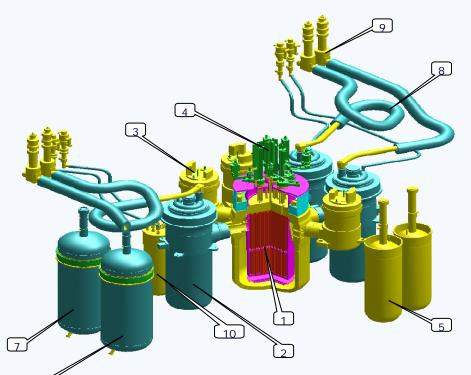
1 Reactor; 6&7 Pressurizers; 2 Steam generator; 8 Steam lines; 3 Main circulating pump; 9 Localizing valves;
