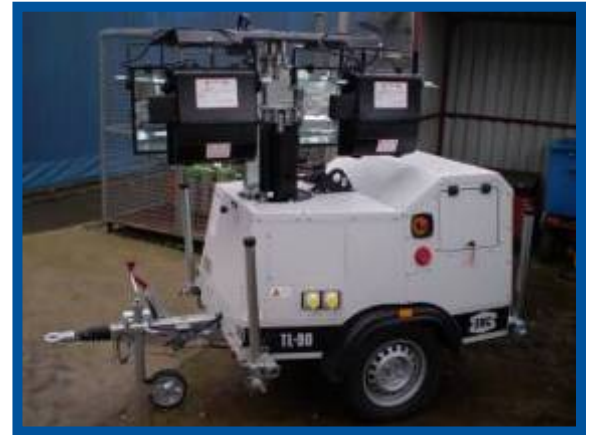
New diesel powered Lighting tower
