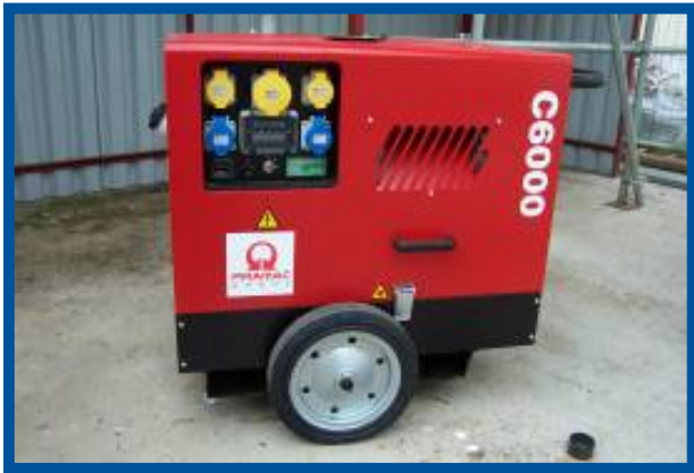
New diesel powered generator
