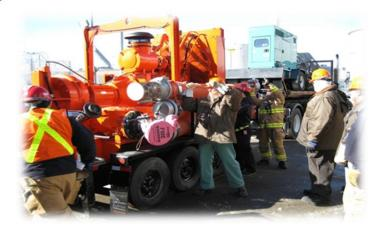
Supply water to CANDU heat sinks with portable pumps
