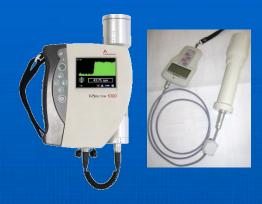
Portable Nal Gamma Detectors maybe used for initial screening of a population for thyroid radioactivity intake.
