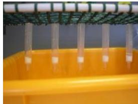
**Sr/matrix separation with a specific resin
