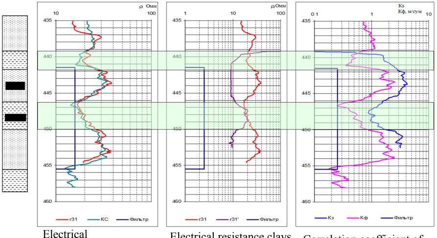
Electrical characteristics of sands, the resulting electrical logging Electrical resistance clays and siltstones before and after acidification
