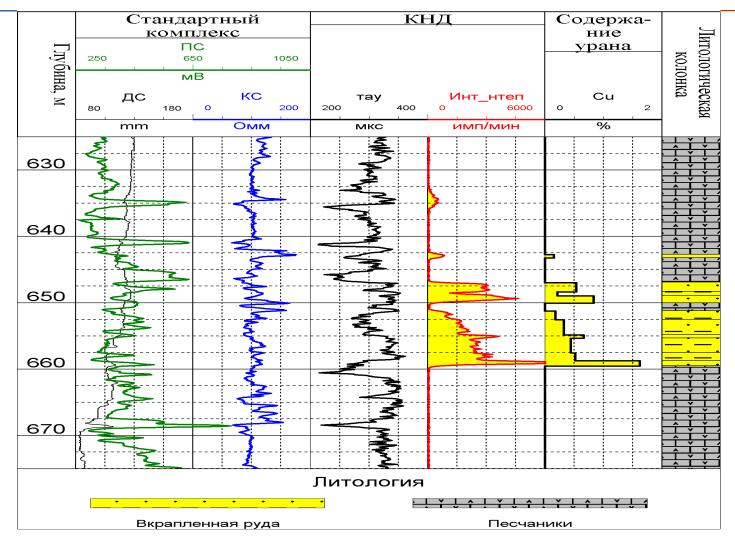
Example of PFN method use in one of deposits in Kazakhstan determine of mass U share taking into account influence of hydrogen content
