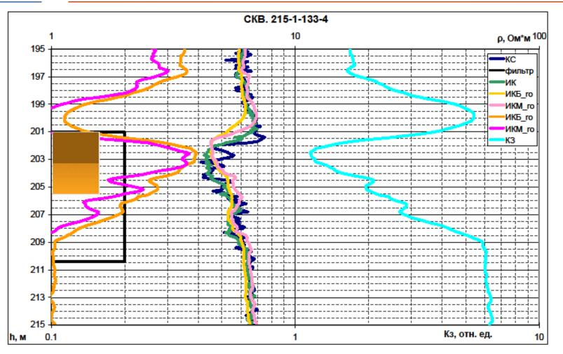
high clayey slightly clayey Induction electric log of two probes (0.5 m and 1 m) before and after acidification
