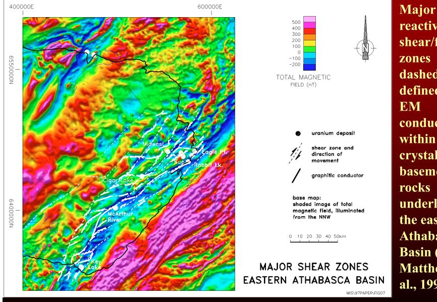
reactivated shear/fault zones (white dashed lines); defined by conductors within the crystalline basement underlying the eastern Athabasca **Basin** (after Matthews et al., 1997).
