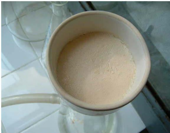
Filtration of Th peroxide precipitate
