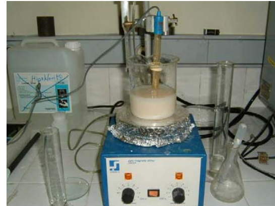
Th peroxide precipitation by H_2O_2 addition
