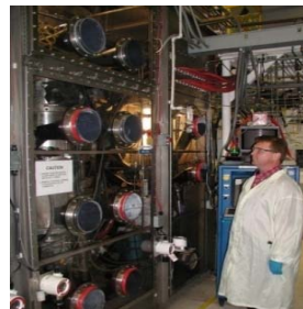
Industrial Scale 6 inch CVD Coating (2 kg charge)
