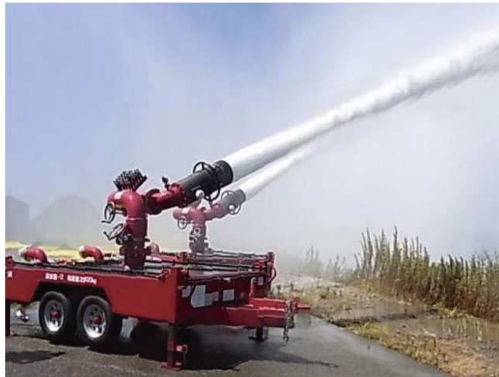
Water-spraying with a large scale bubble water cannon system
