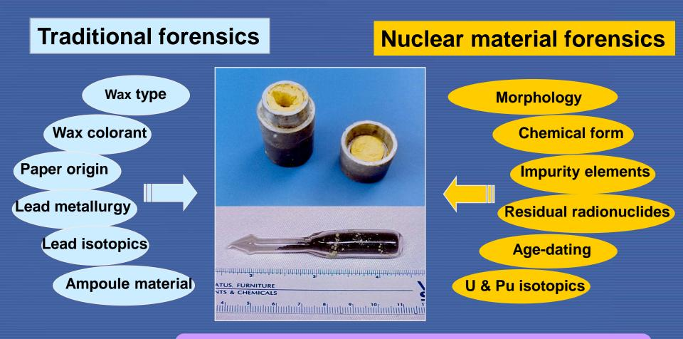
Highly-enriched uranium (~3.96 grams uranium oxide) Trace plutonium (2.8 parts per billion)
