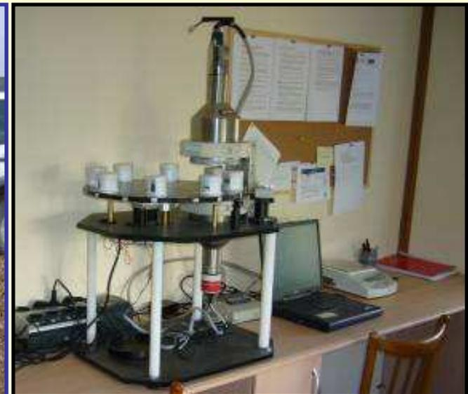
(\*) Has a large-area (12.6 cm), very thin (0.16 cm) sodium iodide detector optimized for low energy photons (~10-100 keV). The emitters such as Pu (13.6 keV) and Am-241 (59.5 keV).
