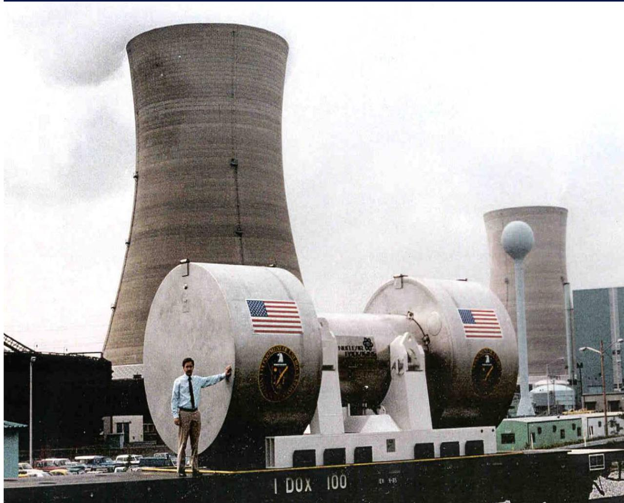
**Shipping casks used to ship fuel debris by rail to the DOE's Idaho National Laboratory**
