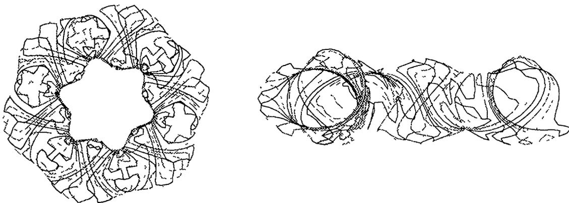
Figure 3: Top view and side view of a set of base case modular coils that can produce the OT7-M4 configuration. Only the front coils are shown in the side view. These coils are clearly too complicated, are too kinky, and offer little access to the plasma, and are only used to generate the external fields for the free-boundary VMEC code.
