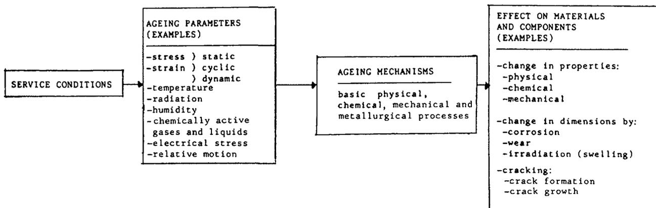
Fig.6.1. Examples of interaction between service conditions and effects on materials and components.
