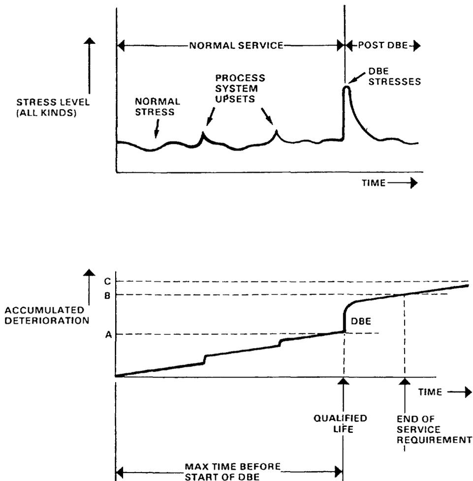
Figure 7.2.4. Accumulated Deterioration Related to Service and Design Basis Event Stresses (seismic, LOCA, MSLB)
