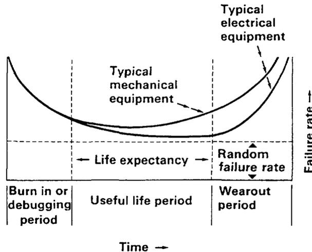
Figure 7.2.3. Time Dependence of Failure Rate
