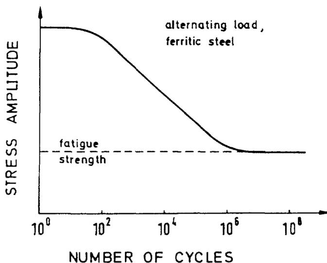
Fig. 6.2.7. Correlation between applied stress amplitude and the number of load cycles to failure (Woehler Diagram)
