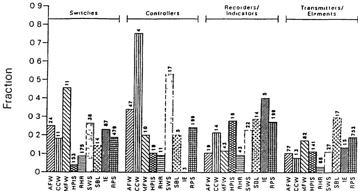
Fig. 5.1.2.3. Relationship of instrumentation component ageing fractions by system.
