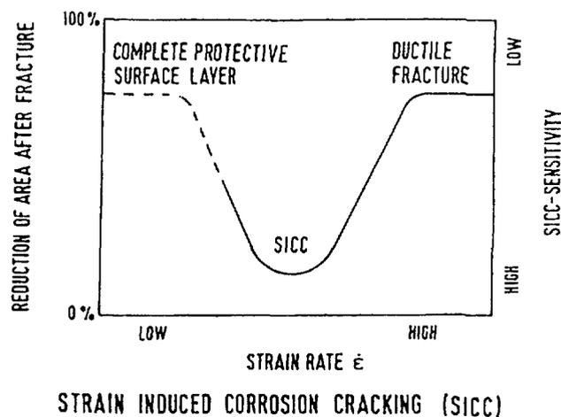
Fig.6.2.10. Effect of strain rate in uniaxial tension test on the reduction of area in corrosive environment
