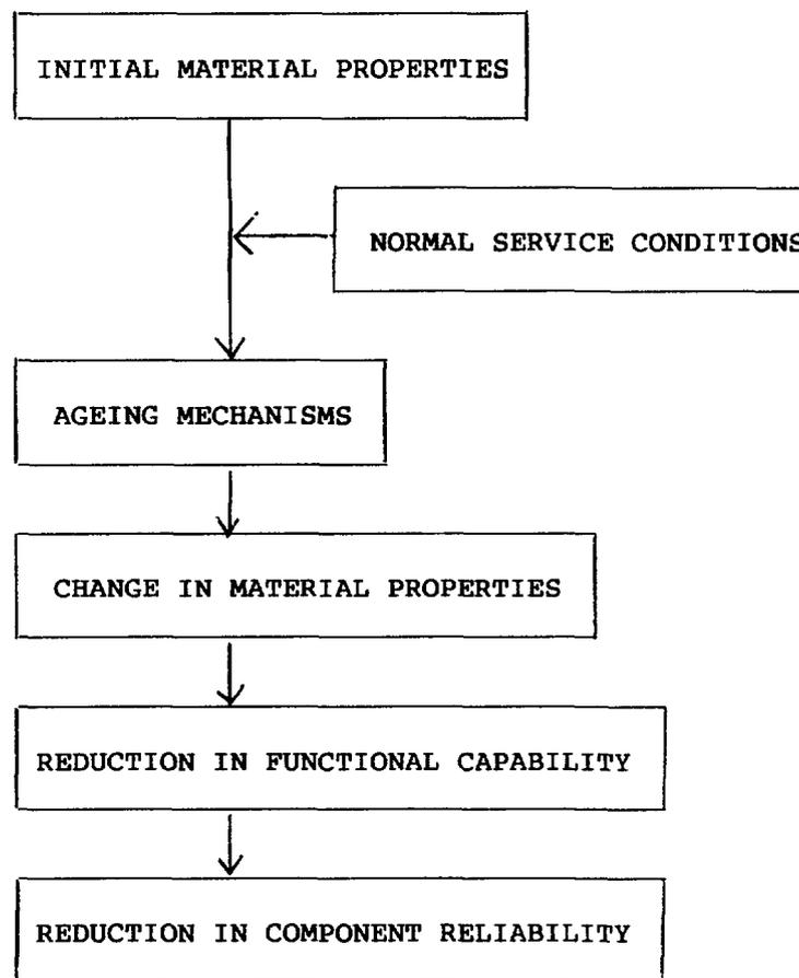
Fig.2.1. Impact of service conditions on material degradation and component reliability.
