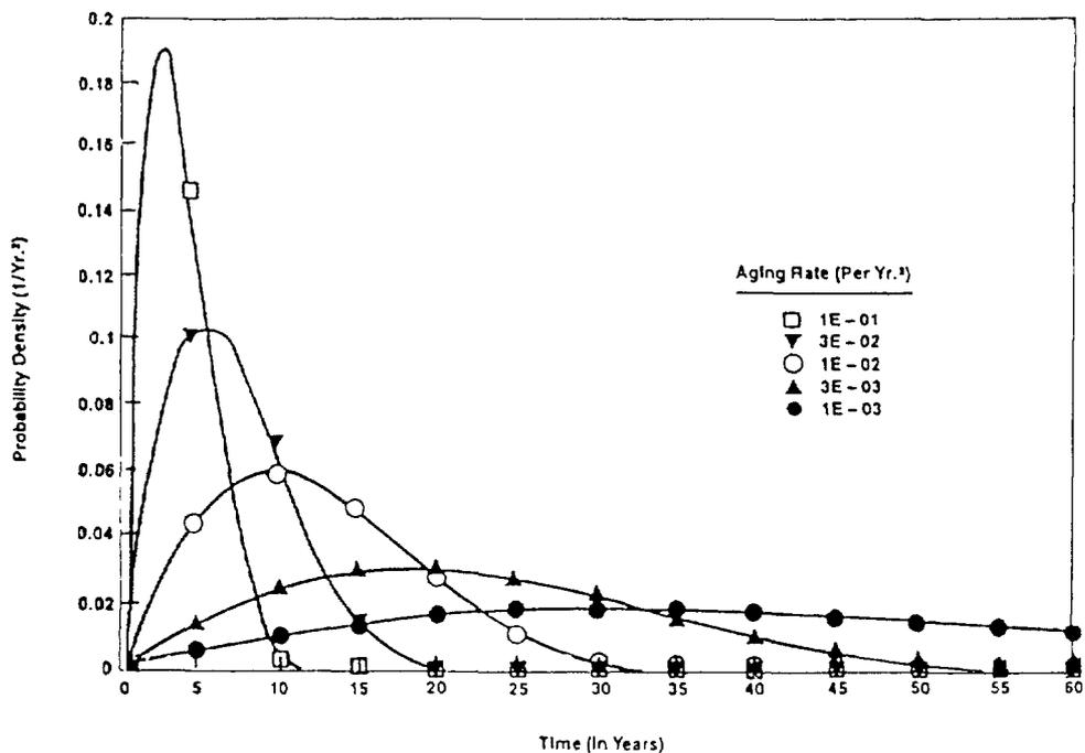
Fig.5.3.4. Time to first failure probability density functions resulting from different ageing rates for the linear ageing model.
