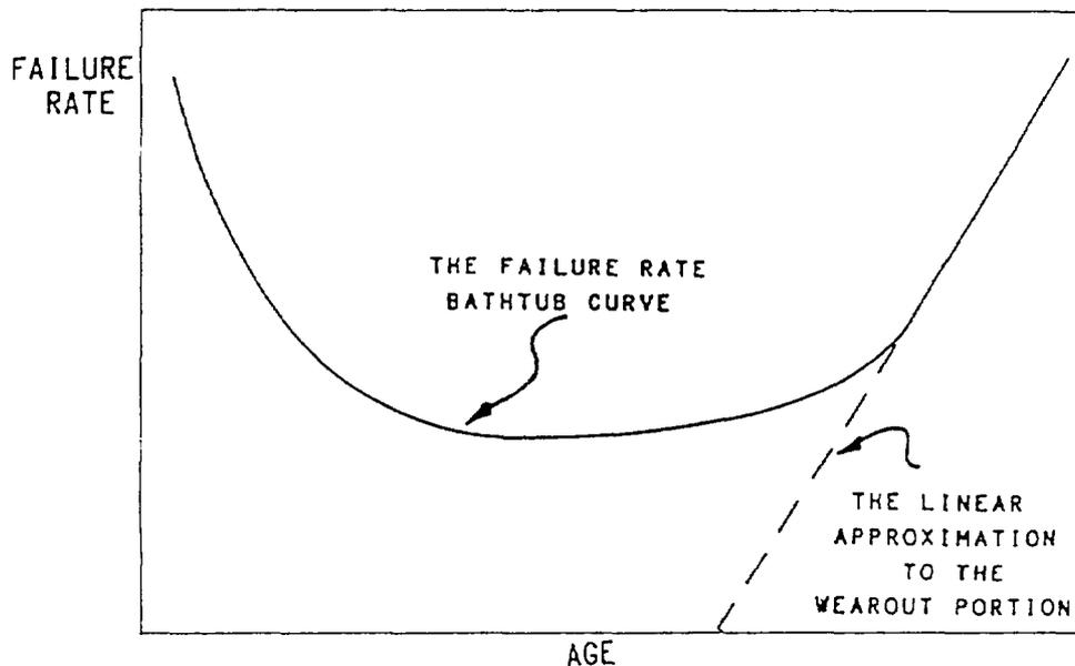
Fig.5.3.3. The bathtub curve and the linear failure rate fit.
