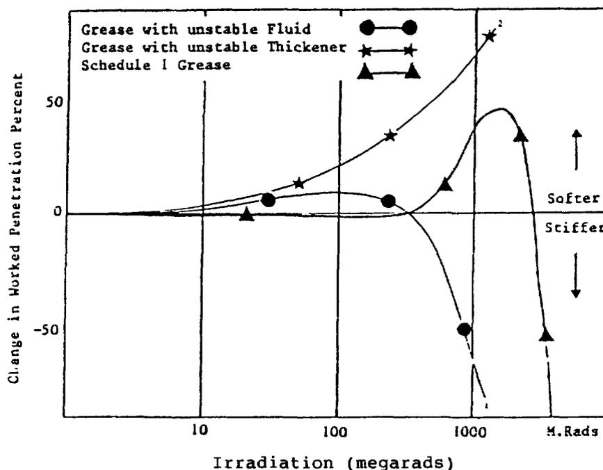
Fig. 6.4.4.1. Effect of radiation on greases of various stabilities.
