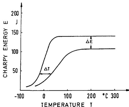
Fig. 6.2.3. Change in material toughness due to neutron irradiation measured in Charpy-V notch impact test
