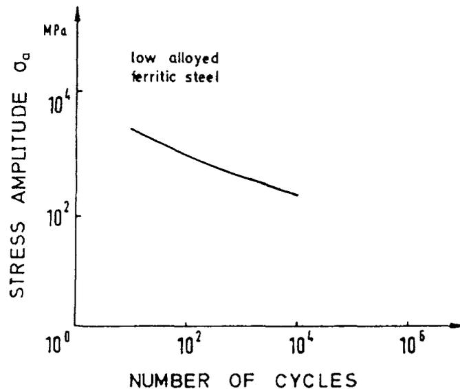
Fig. 6.2.8. Design curve for allowable strain amplitude as a function of the number of cycles in the low cycle regime
