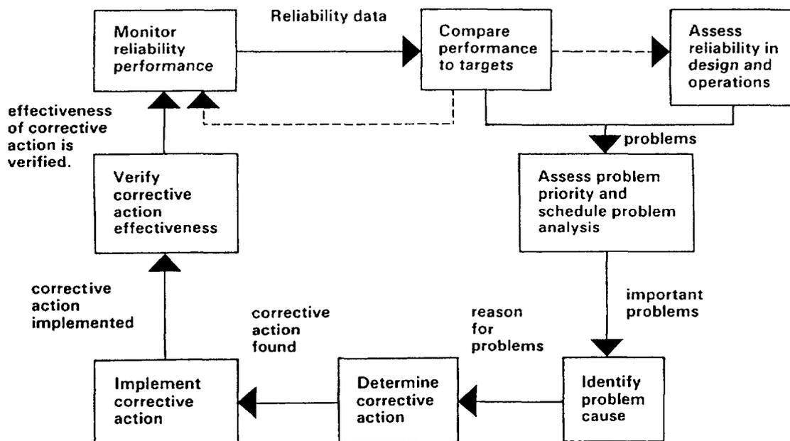
Figure 7.2.5. System Reliability Monitoring Process
