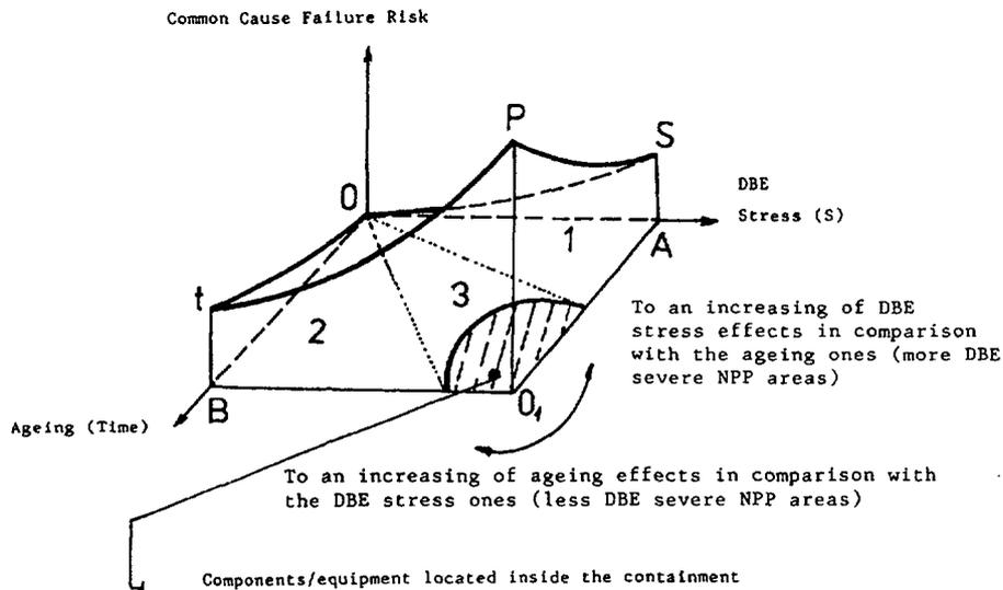
Fig.A.1. Risk of common cause failure: a function of DBE stress and ageing.
