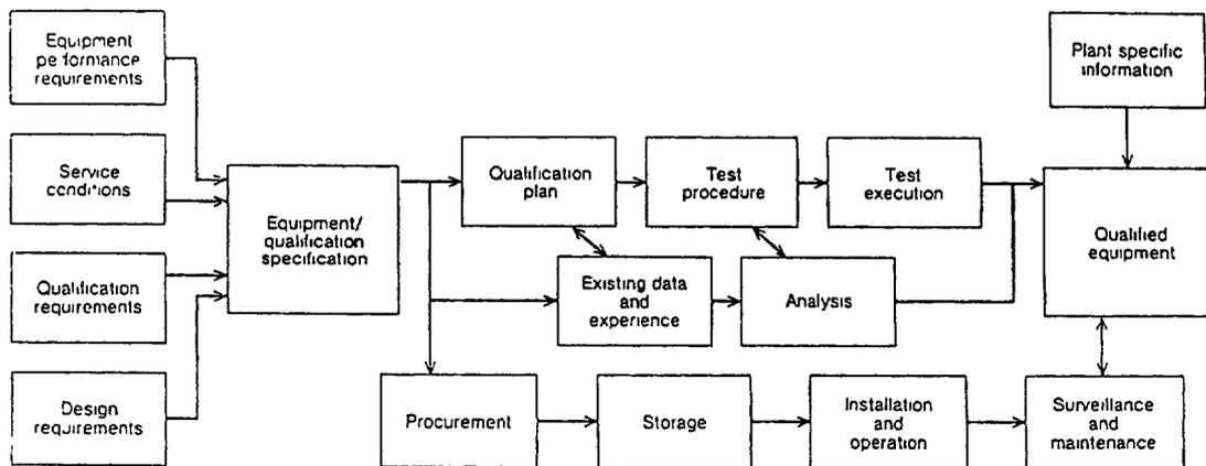
Fig.4.2. Equipment qualification process - block diagram.
