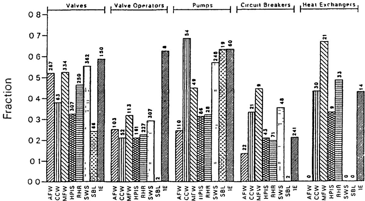
Fig.5.1.2.2. Relationship of component ageing fractions by system.
