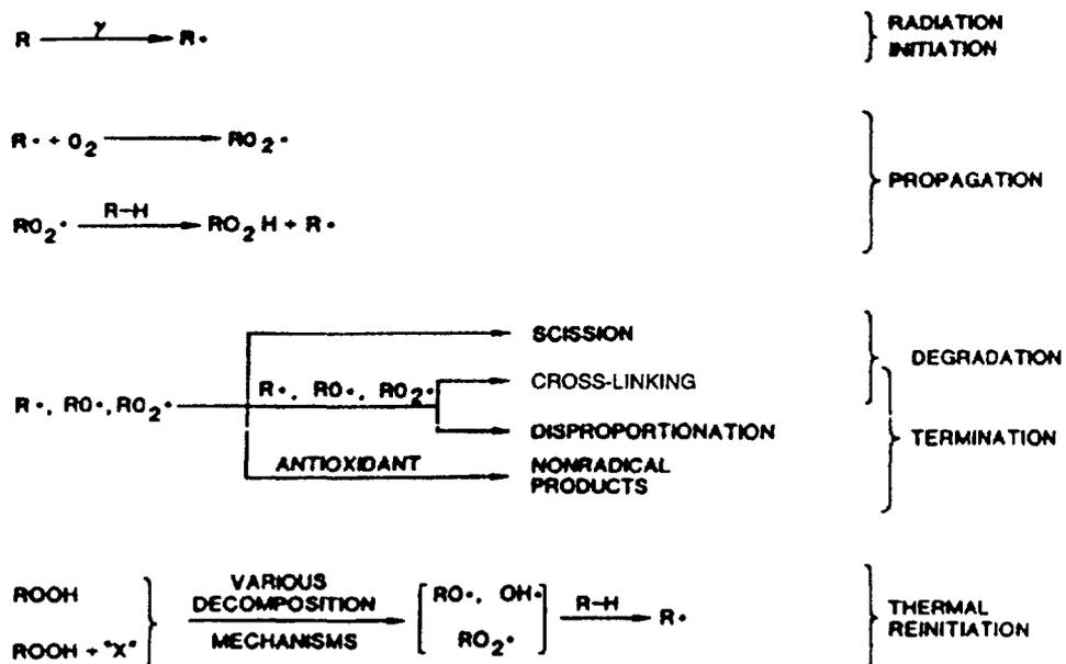
Fig 6.4.3.2.1. Chemical mechanism for radiation induced oxidation.
