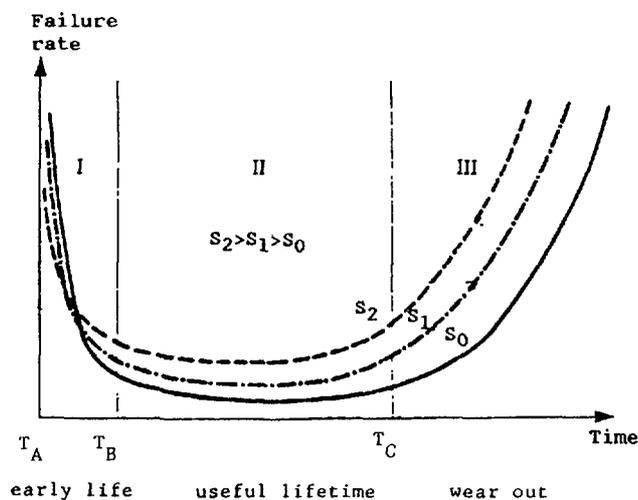
Fig.A.2. Bathtub shaped reliability curve.
