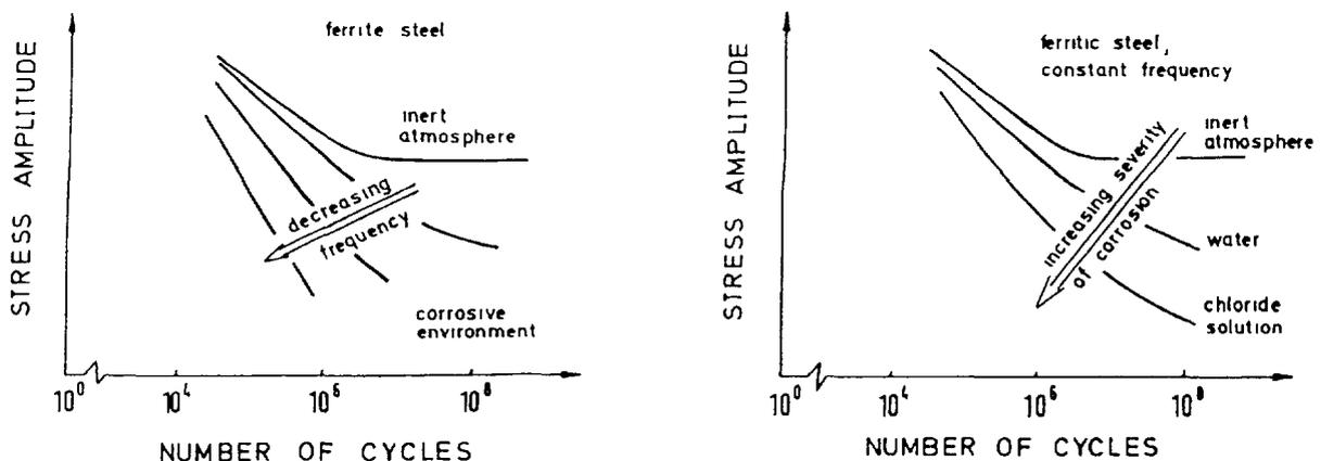
Fig. 6.2.11 a and b. Effect of frequency on the number of cycles to failure in corrosive environment
