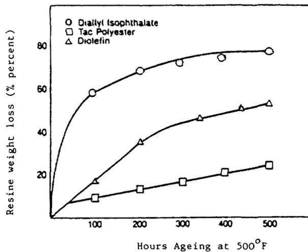
Fig.6.4.5.1. Percentage resin weight loss of style-120 glass fabric laminated during ageing at 500°F.
