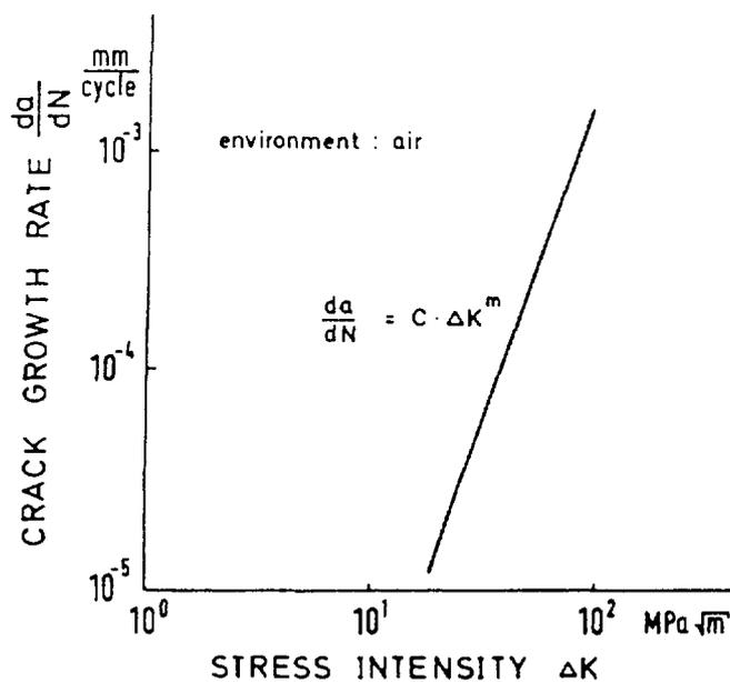
Fig. 6.2.9. Cyclic crack growth rate as a function of stress intensity amplitude
