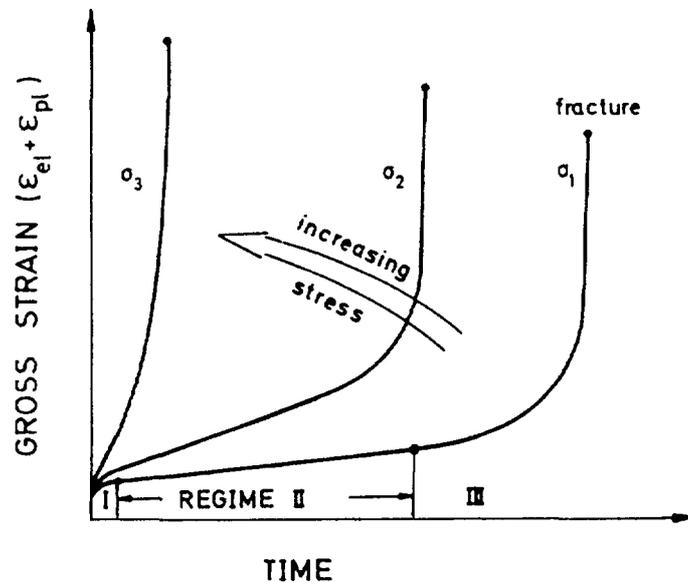
Fig. 6.2.6. Typical creep behavior of steels governed by different mechanisms in regimes I through III
