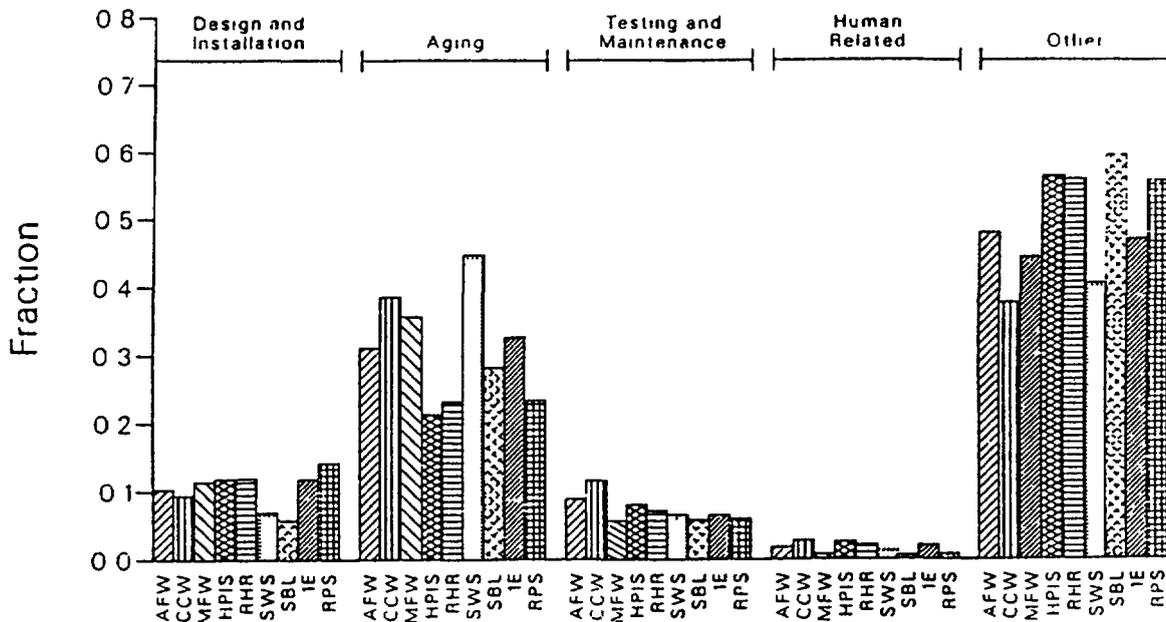
Fig.5.1.2.1. Relationship of failure category fractions by system.
