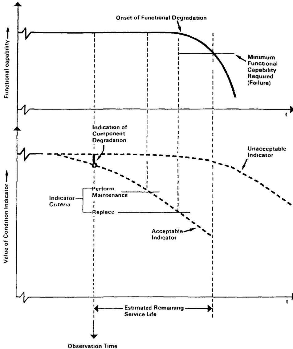
Fig. 7.2.1. Use of Condition Indicators for Condition Monitoring
