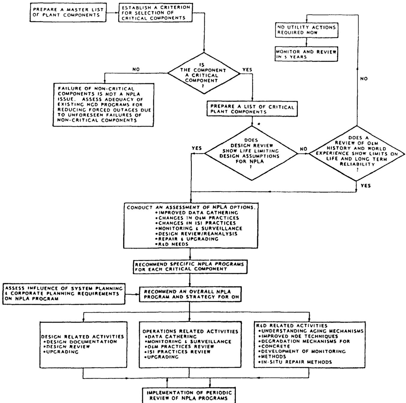
Fig.8.5. Methodology for a nuclear plant life assurance (NPLA) programme.
