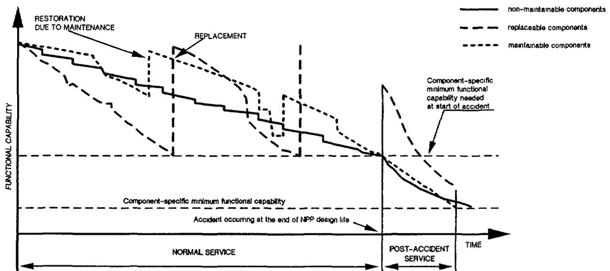
Fig.4.1. Qualitative picture of functional capability changes of different types of components during normal operation and following an accident occurring at the end of NPP design life.
