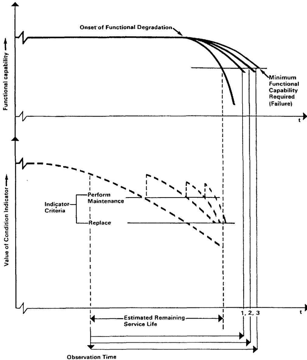
Fig. 7.2.2. Effects of Preventive Maintenance on Functional Capability and Remaining Estimated Service Life
