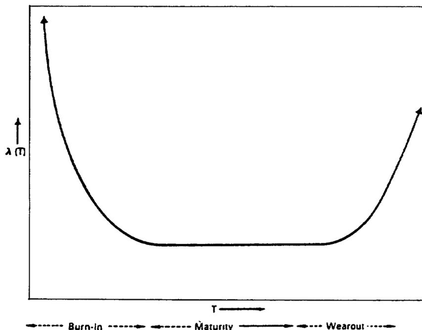
Fig.5.3.1. Example of a failure rate curve.
