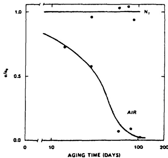
Fig. 6.4.3.2.2. Tensile elongation results for PE insulation as a function of ageing time at 5 krad/h, 80°C in atmospheres of air and  $N_2$  [46].
