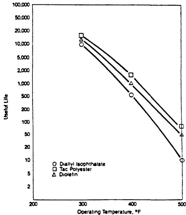
Fig.6.4.5.2. Thermal life curves of style-120 glass fabric laminated feeddomes, based on 10% maximum possible resin weight loss for a useful life.
