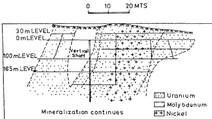
FIG. 3. A longitudinal section of the Jaduguda Mine.
