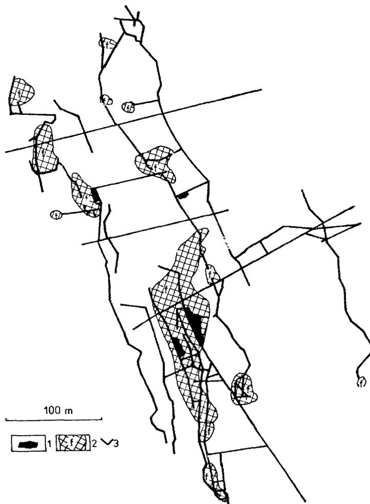
FIG. 5. Level plan of the Kletno mine. 1. aggregates of polymetallic uranium mineralization; 2. pots of fluorite; 3. drifts.
