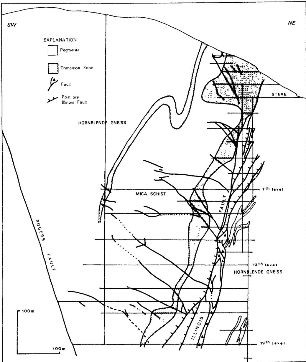
FIG. 2. Cross section of the Schwartzwald uranium deposit, showing mine workings and geology. From Wallace et al. (1).
