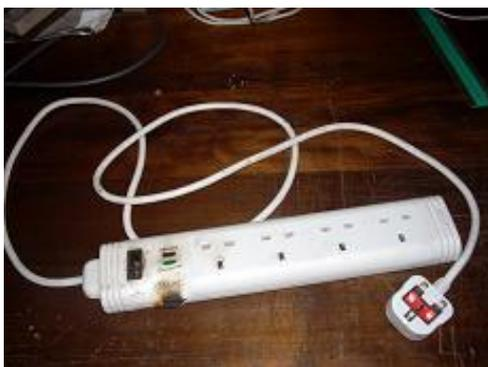
*Fig. 4 Power distribution board failure*
