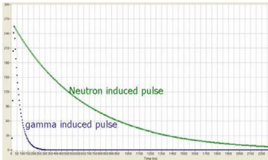
*Fig. 2 Normalized plot of light decay from neutron and gamma induced scintillation pulses*
