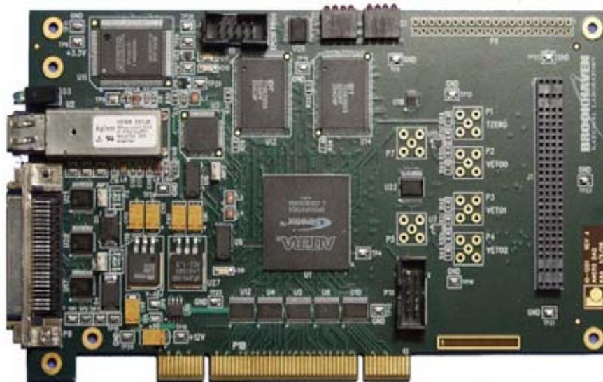
*Fig. 3 The PCI data capture and timestamping module*
